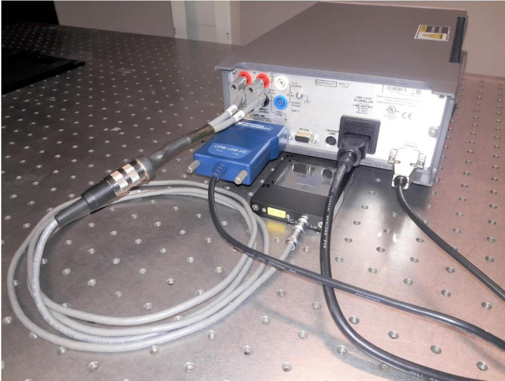
1. Connect the round Amphenol connector of the Reference Cell cable (90021927) into the round Amphenol connector of the 91150V-CBL (Cable - Ref Cell to Keithley).
