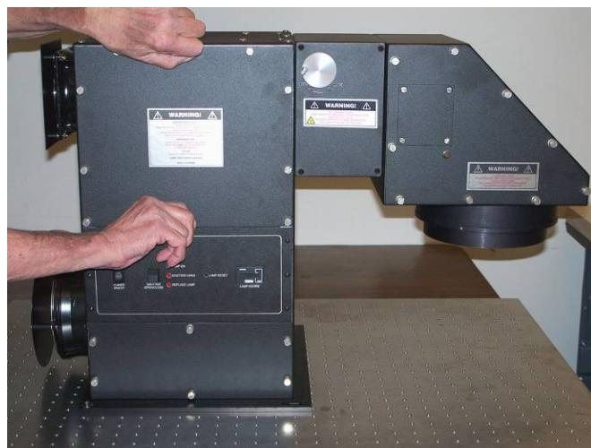
*Photo 21: Removing the lamp access panel*
