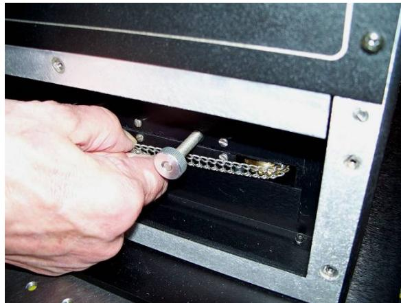
*Photo 28: Adjustment using the ladder chain*
