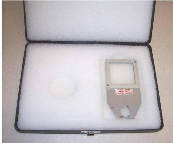
*Photo 3: Air mass filter assembly (stored in case)*
