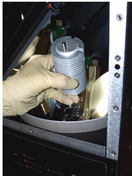
*Photo 25: Heat sink unscrewed from socket*
