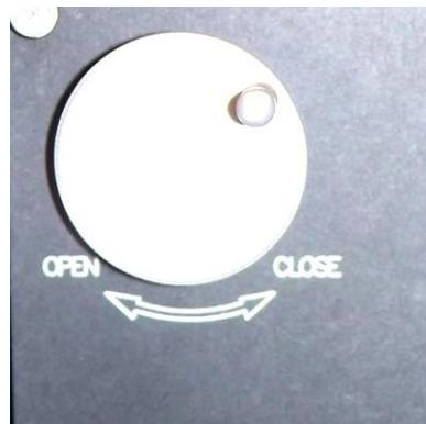
4. To use the partial SUN attenuator, adjust the knob in either direction to attain the desired irradiance level when the solar simulator is turned on. (*Note: In order to verify the desired irradiance level has been reached, a calibrated reference cell or any irradiance measuring device should be used. Relying on the number of turns or the knob orientation for any particular level of irradiance will not guarantee repetitive results.*)
