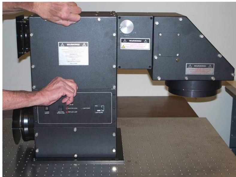
*Photo 12: Removing the lamp access panel*
