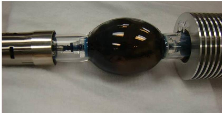
*Photo 30: Lamp run under reverse polarity*
