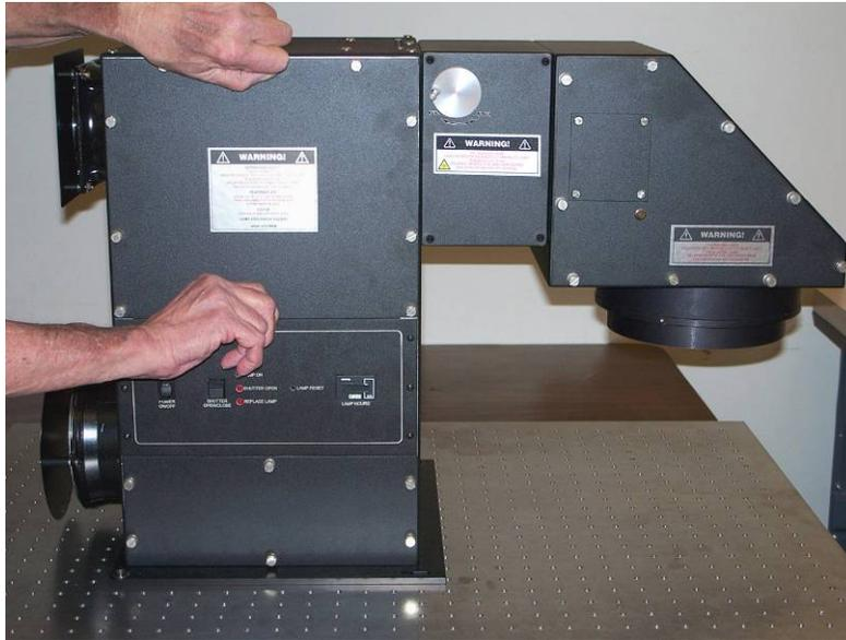
*Photo 12: Removing the lamp access panel*
