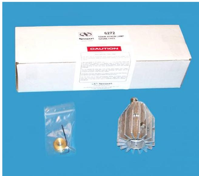
*Photo 2: Lamp and heat sink (with packing crate)*
