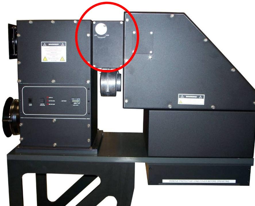
As shown above in the red circle, the partial SUN attenuator fits in the middle section of class 3A solar simulator housings.
