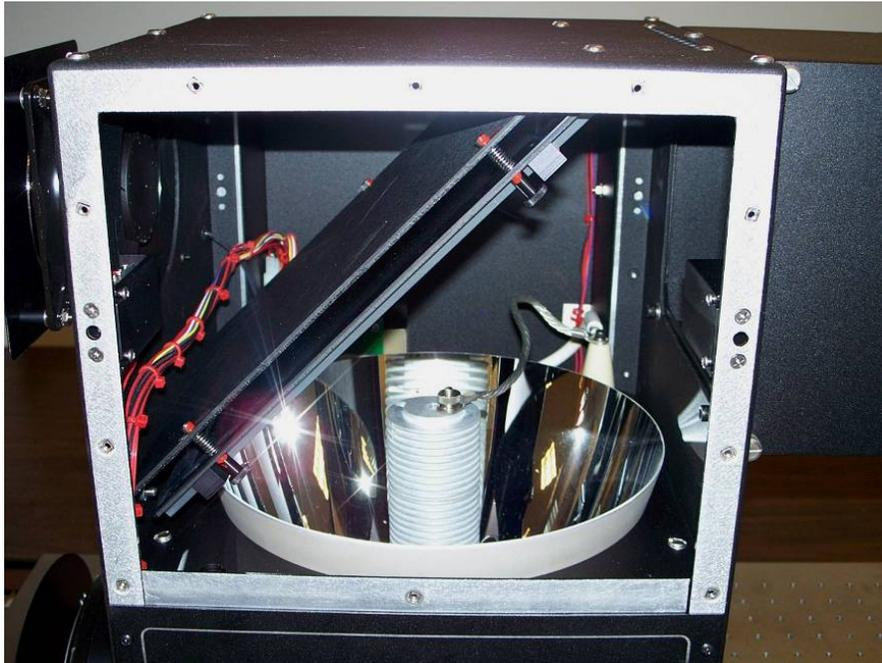
*Photo 22: Lamp access panel removed*
