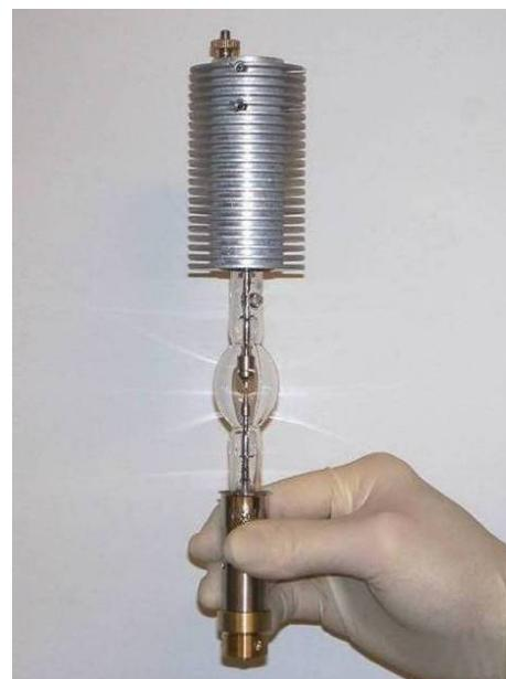
Figure 2: Installing the 450W Lamp
