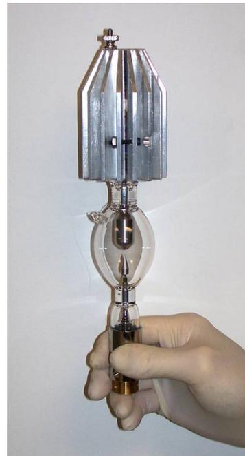
Figure 4: Installing the 1.6kW Lamp
