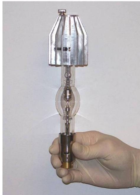
Photo 15: 1kW lamp with heat sink attached
