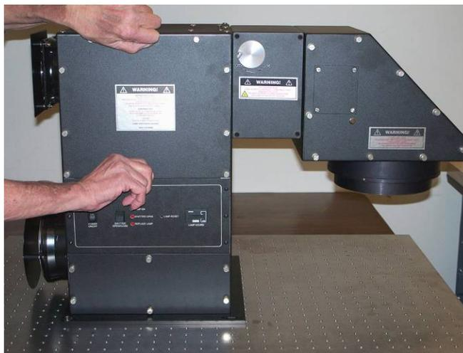
*Photo 21: Removing the lamp access panel*
