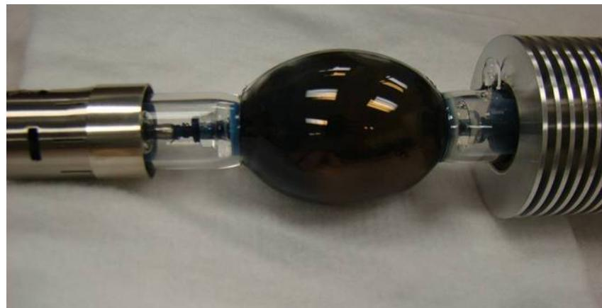
*Photo 30: Lamp run under reverse polarity*
