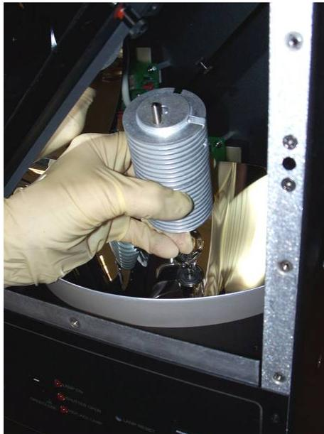
*Photo 25: Heat sink unscrewed from socket*
