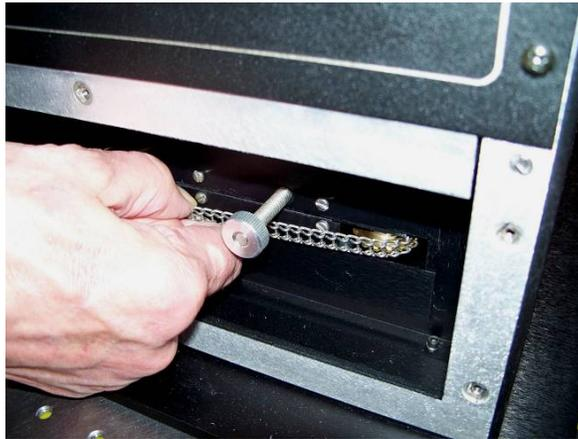
*Photo 28: Adjustment using the ladder chain*
