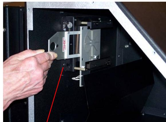
Photo 8: Filter Installed 2x2 and 4x4 models
