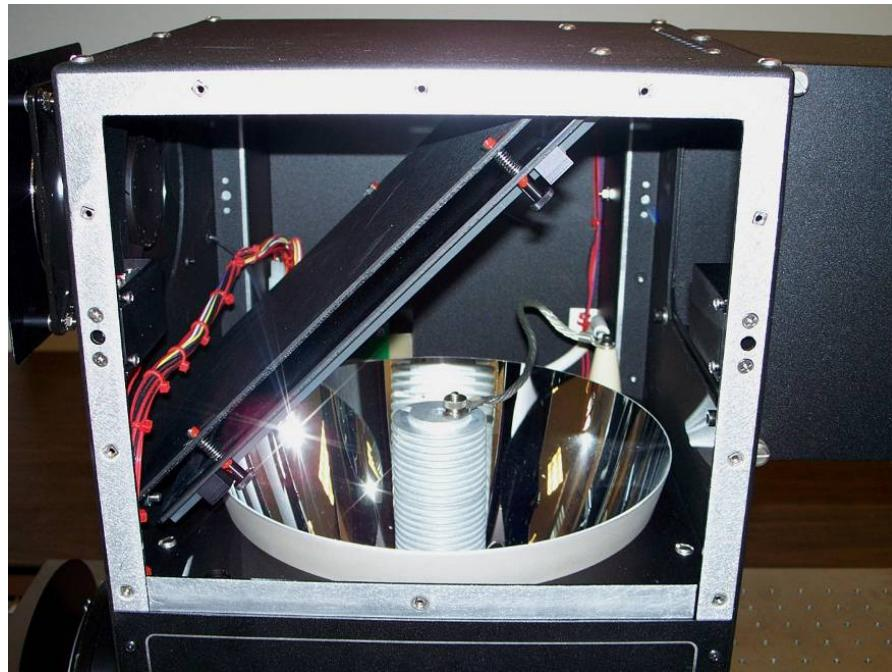
*Photo 22: Lamp access panel removed*
