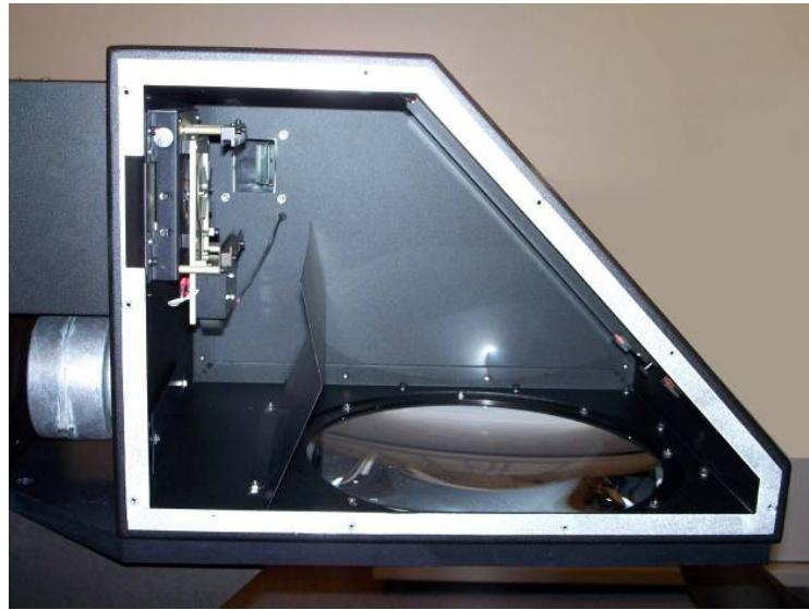
*Photo 10: Output assembly, side cover removed*
