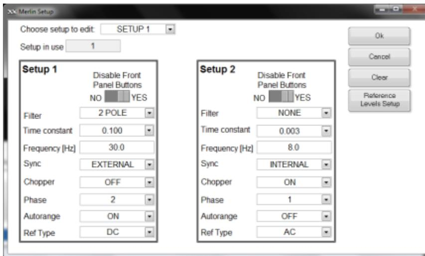
Figure 130: Merlin Operating Parameters Setup, Single Channel
