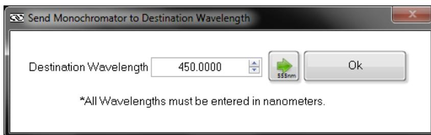
Figure 114: MS257 Selecting a Monochromator Output Wavelength
