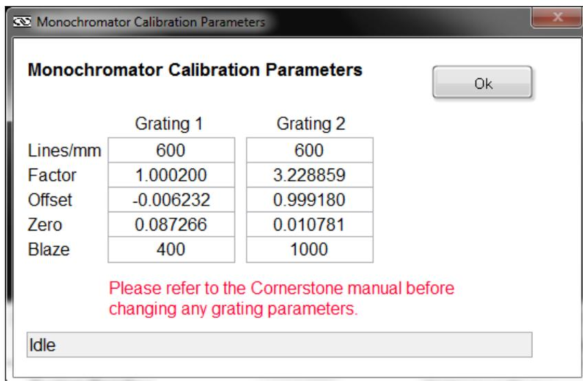
Figure 99: Monochromator Calibration Parameters
