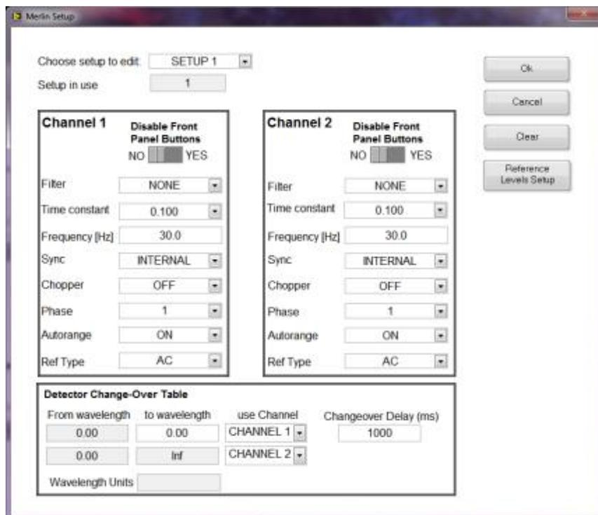
Figure 131: Merlin Operating Parameters Setup, Dual Channel
