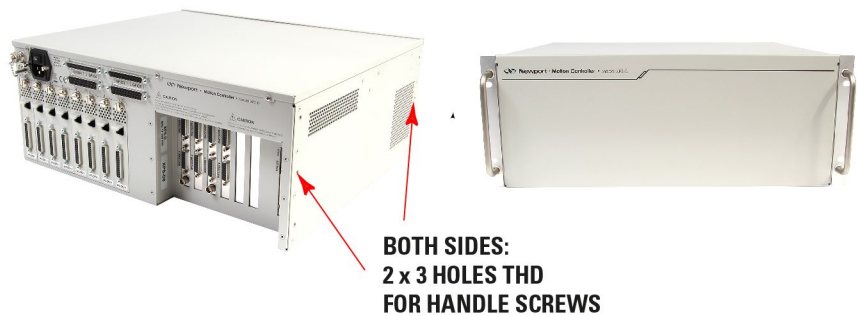
Figure 11: Installing handles
