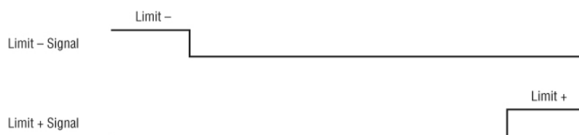
Figure 28: Limit - and Limit + TTL input signals.
