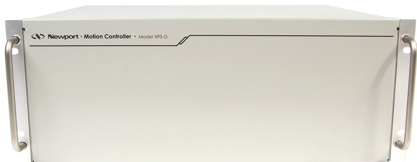
Figure 7: Front panel of XPS Controller/Driver.
