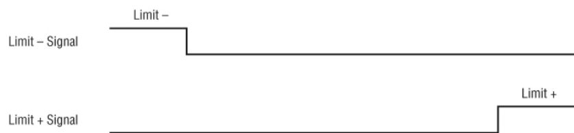
Figure 28: Limit - and Limit + TTL input signals.
