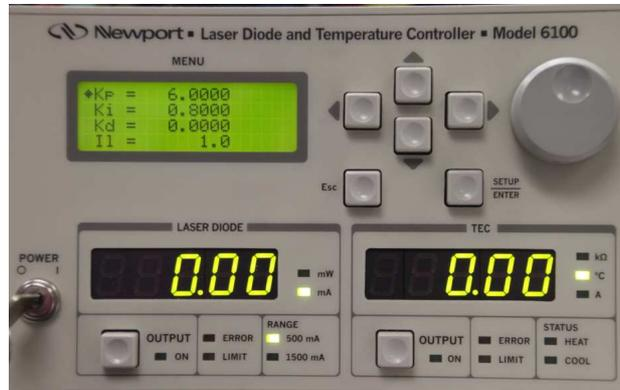
Make changes using the arrow keys and dial as needed, by pressing the right or left arrow keys to get to the digit you wish to change, then use the up or down arrow (or dial) to make the change.
