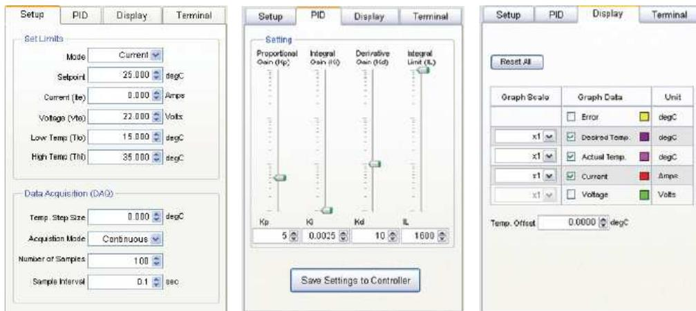
Begin by setting up the Display tab. Here you can choose which parameters you would like to monitor. We suggest the Current, Voltage, Desired Temp (Set Point) and Actual Temp. The pre-assigned curve colors cannot be changed.
