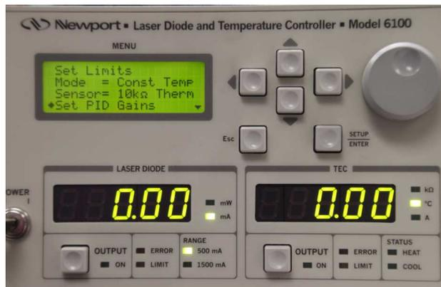
In the next window, use the arrow keys to select Customize Gain, and press the SETUP/ENTER button again.
