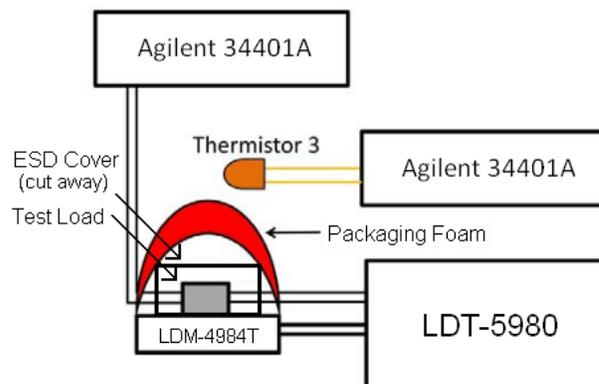
**Figure 2: Experimental setup for temperature stability testing**
