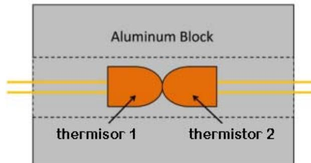
**Figure 1: Internal view of the test load showing adjacent thermistors**
