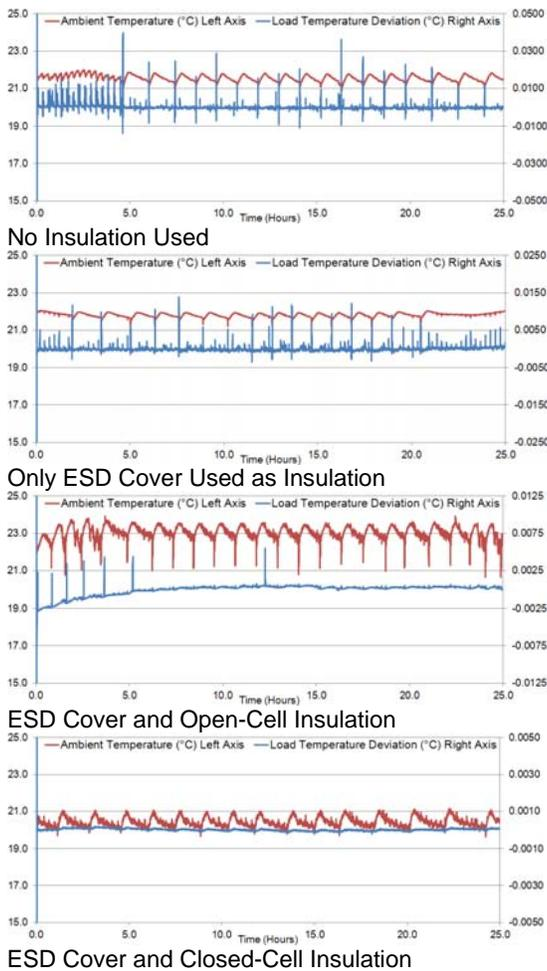
**Figure 5: Stability with different insulation**
