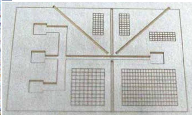
Cutting and structuring of polymers (sensors and microfluidic devices) using a high-power, ultrafast industrial laser.
