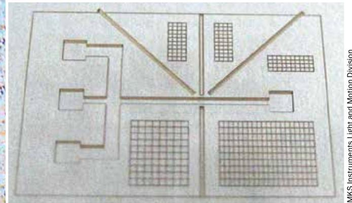
Cutting and structuring of polymers (sensors and microfluidic devices) using a high-power, ultrafast industrial laser.
