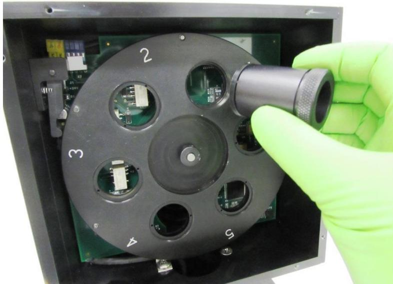
**Figure 37: Filter Wrench Removing Retaining Ring**
