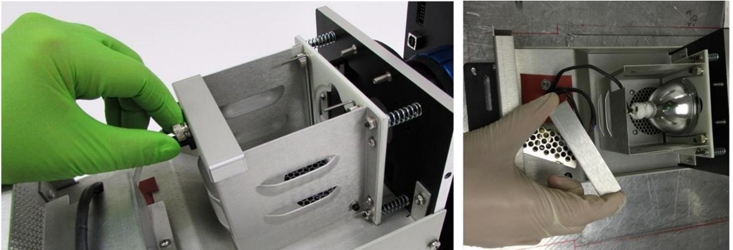
**Figure 11: Remove Lamp Cable Holder**
