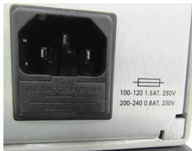
Figure 56: Fuse Compartment
