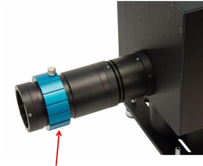
Figure 33: Collimating Lens Adjustment
