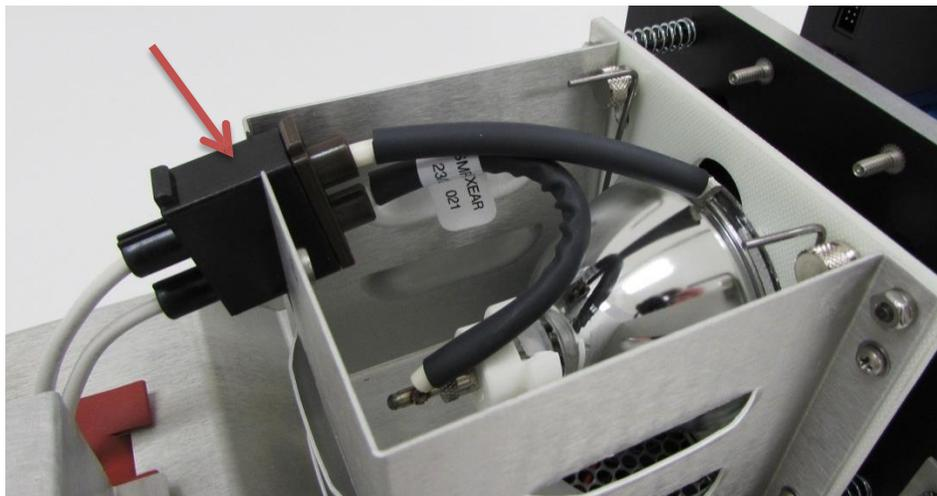
**Figure 17: Connect Lamp Wiring**
