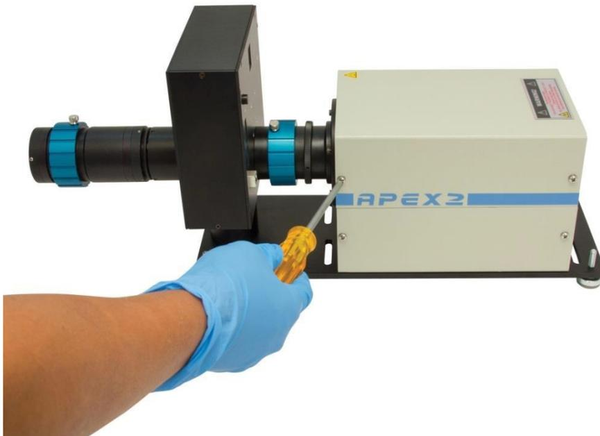
**Figure 9: Remove Top Cover Screws**
