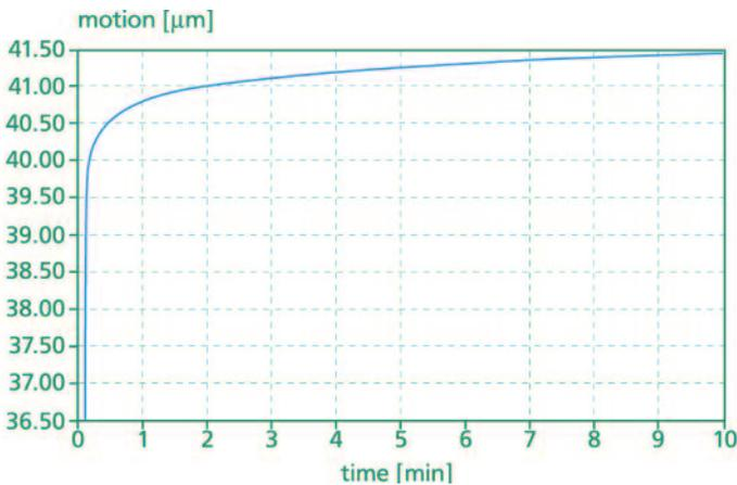
**Figure 1.18** Creep of a PU 40
