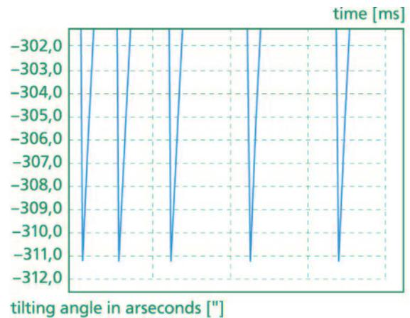
**Figure 1.19** Repeatability of a position with periodic motion of a mirror mount
