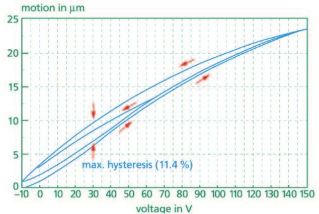
**Figure 1.7** Typical hysteresis curve of a multilayer piezostack
