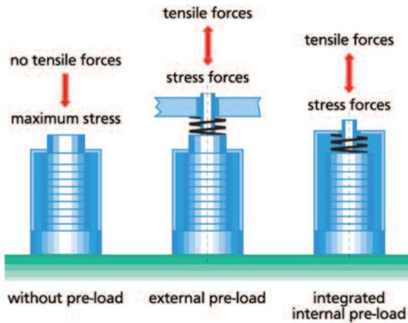
**Figure 1.3** Piezos with and without preload
