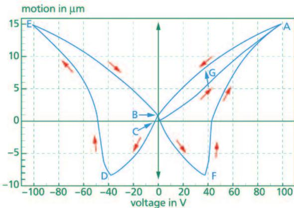
**Figure 1.6** Via the applied voltage, the motion of the element will follow the points ABCDEF.
