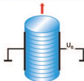
**Figure 1.2** Construction of a piezostack
