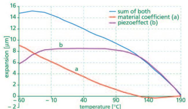
**Figure 1.15** Example of temperature dependence of multilayer ceramic  $L_{piezo} = 18mm$  at room temperature.
