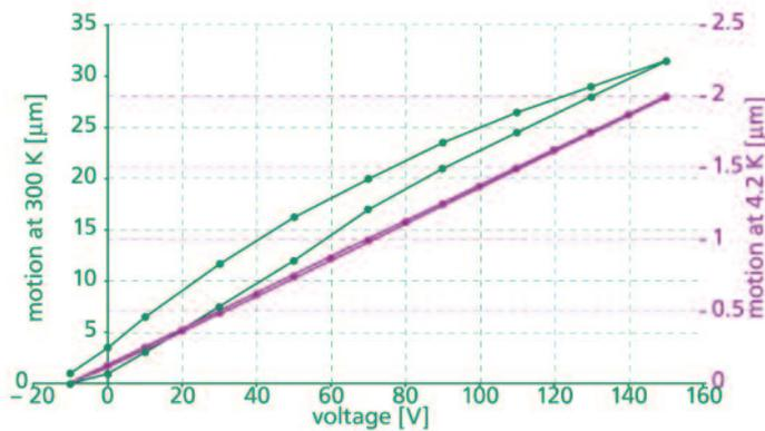
**Figure 1.16** Hysteresis curve of a NPA 25 element at room temperature and at 4K.
