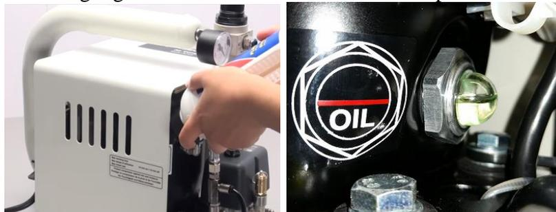
Figure 3 Add oil and check oil level
