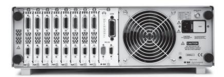
The back panel of the LDC-3908 instrument, with 8-channel full capacity module loading. Offering secure and flexible module population, customized to fit your testing needs. Standard 1 MHz modulation port and GPIB / RS232 remote terminals expand upon its application and control.
