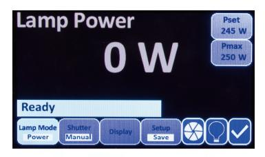
The OPS Series power supplies allow the lamp to be operated in power, current, and intensity control modes.
