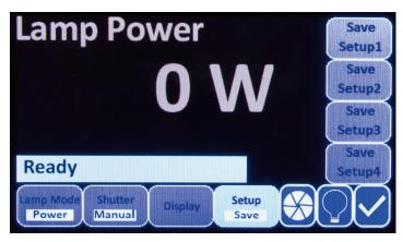
The OPS model power supplies are capable of storing up to four Setups.
