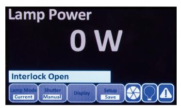
Newport's Oriel Power Supplies have a safety interlock feature which must be satisfied before the power supply will power the lamp and which, if broken during operation, will disable the power supply. Overheating of the housing or accidental opening of the door will automatically shut down the power supply.
