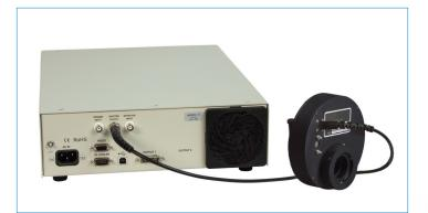
The shutter control feature of the OPS model power supply is useable in power, current, and intensity control modes. Any shutter which responds by opening or closing when receiving a TTL signal can be controlled by the OPS Power Supplies. This includes Oriel's model 71445 low-cost TTL shutter and the shutters designed into the Oriel Solar Simulators.
