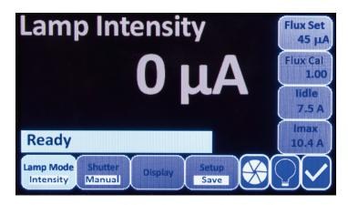
Intensity Mode requires the use of the LIK-LMP light intensity controller kit, also made by Oriel Instruments. When operating in the lamp in Intensity Mode, the user can adjust the Flux Set parameter until the desired output intensity of the lamp is attained.
