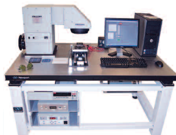
Complete Oriel I-V Tester setup on a workstation. Solar simulator and workstation are sold separately. Computer is not included in the Station.
