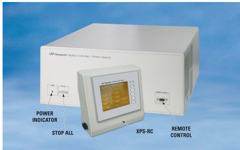
Figure 7: Front Panel of XPS Controller/Driver.
