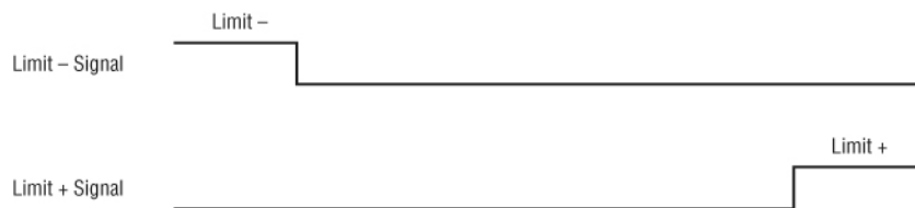
Figure 77: Limit and Limit TTL Input Signals.
