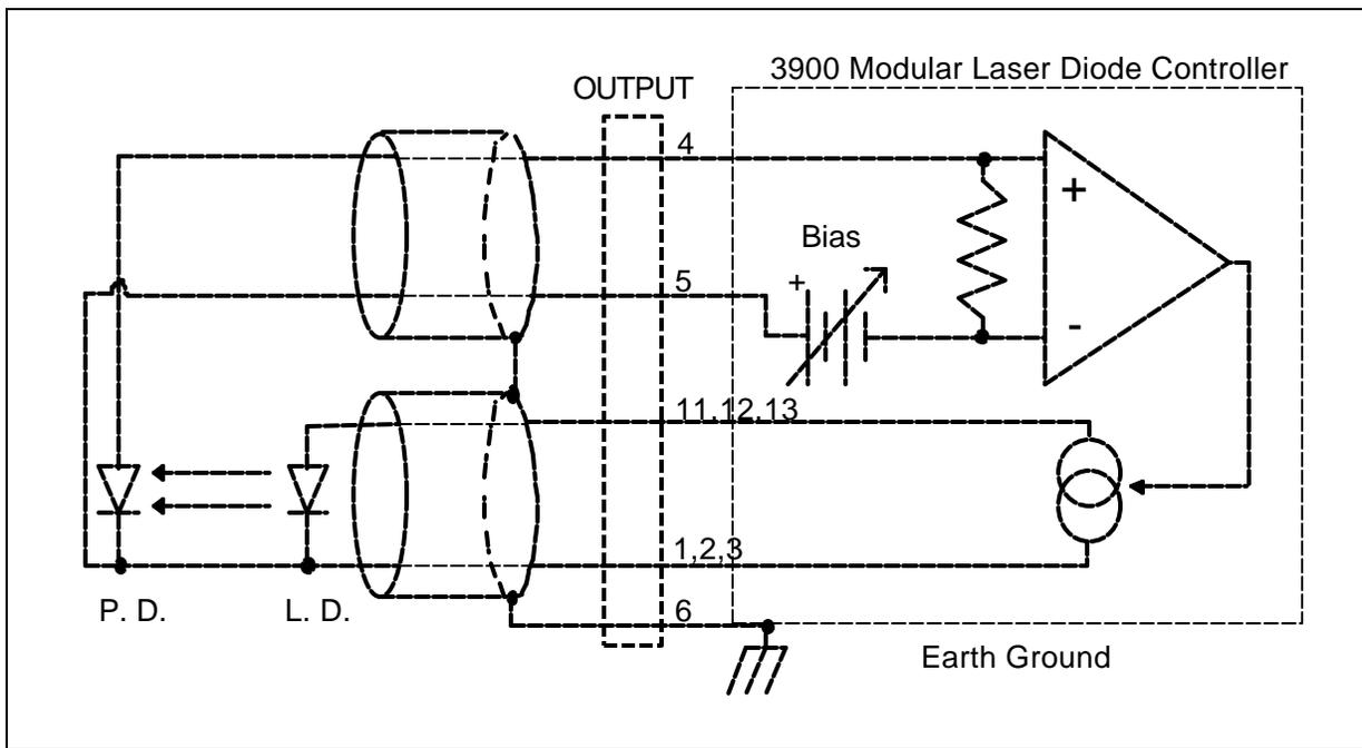
Figure 4.3A Common Laser Cathode - Photodiode Cathode
