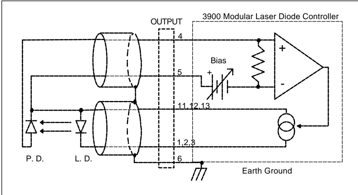
Figure 4.3C Common Laser Anode - Photodiode Cathode
