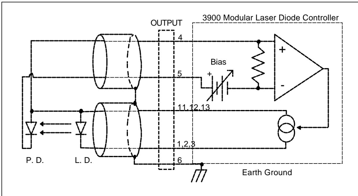
Figure 4.3D Common Laser Anode - Photodiode Anode
