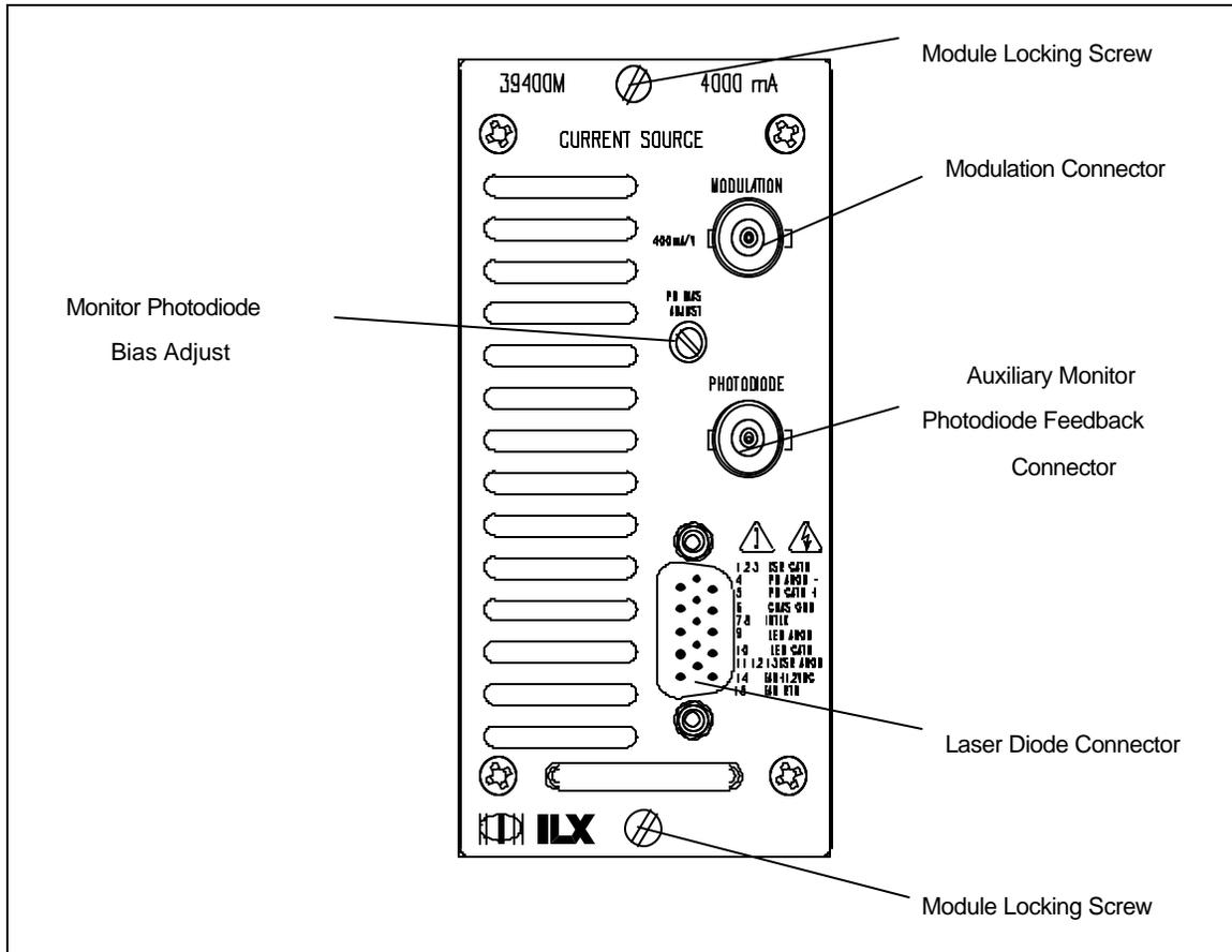
Figure 4.1 CSM-39400M Back Panel
