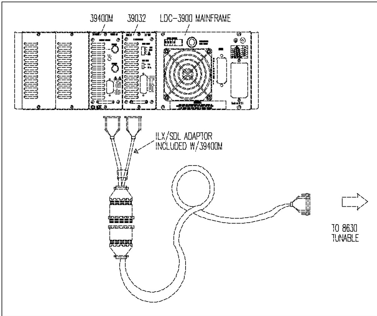
**Figure 4.5 LDC-3900/Tunable Laser Configuration**
