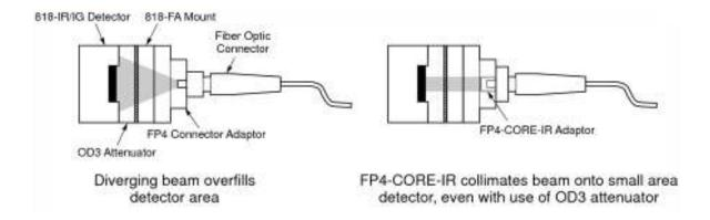
For the distance calculations involving the connector adapters, it is assumed that the tip of the ferule is flush with the outer shoulder of the connector adapter.
