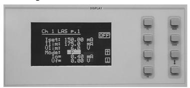
Select the Mode parameter by pushing the (DISPLAY) UP/DOWN ARROW keys until the Mode parameter is highlighted. Repeatedly pushing the (ADJUST) UP/DOWN ARROW keys or turning the ADJUST knob will cycle through the Constant Current low bandwidth (Ilbw), Constant Optical Power (P), Constant Current high bandwidth (Ihbw), and Photodiode Current (Ipd) control modes. Set the LDC-3916330 Series Controller Module in Constant Optical Power mode by selecting the P mode.
