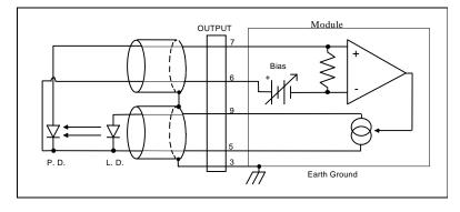
Figure 2.1 Common Laser Cathode - Photodiode Cathode
