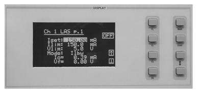
Next, select the Iset parameter on the setup menu using the (DISPLAY) UP/DOWN ARROW keys. This parameter sets the laser current source drive value when in Ilbw or Ihbw modes. Enter 150 mA using the numeric keypad, the ADJUST knob, or the (ADJUST) UP/DOWN ARROW keys. Push the ENTER key to store the value in memory within three seconds after entering the value using the numeric keypad, or it will revert to the old value.
