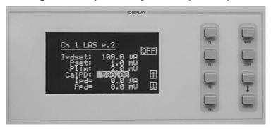
The correct responsivity value (CalPD) must be set for the constant power mode to operate properly. To do this, select the CalPD parameter, and adjust it to the correct value. The CalPD units are  $\mu A/mW$ .
