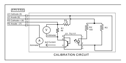
Figure 5.1 I<sub>PD</sub> Calibration Circuit
