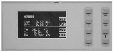
To enter the setup menu, push the CHAN key, which displays the channel menu. Select the correct channel number at the top of the display by pushing the (ADJUST) UP/DOWN ARROW keys or turning the ADJUST knob. For the 3916332/334 modules, push the DISPLAY LAS soft key (F2) to enter page 1 of the laser setup menu. (See image above.)
