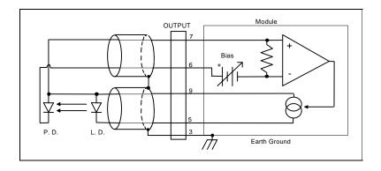
Figure 2.4 Common Laser Anode - Photodiode Anode
