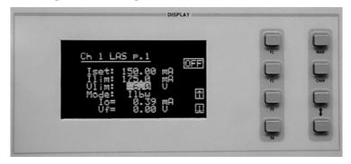
Next, select the laser voltage limit (Vlim) parameter using the (DISPLAY) UP/DOWN ARROW keys. Adjust this value to your desired laser voltage limit. The voltage limit also protects your laser by shutting off the source driver if the laser
