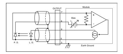
Figure 2.2 Common Laser Cathode - Photodiode Anode
