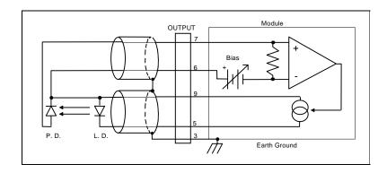
Figure 2.3 Common Laser Anode - Photodiode Cathode
