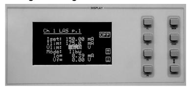
Select the voltage limit (Vlim) parameter and adjust it to 6 volts in the same manner as described above. The voltage limit also protects your laser by shutting off the source driver if the laser voltage exceeds the Vlim value. The Vlim value should be set slightly above the operating voltage of the laser diode to provide maximum protection.
