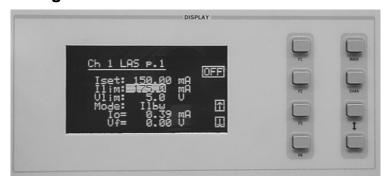
Now select the current limit (Ilim) parameter using the (DISPLAY) UP/DOWN ARROW keys. Adjust the value to 175mA. The current limit protects your laser by never allowing the laser drive current to exceed the Ilim value independent of the current set point and the controller mode (Constant Current or Constant Power).
