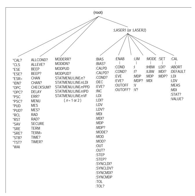
Figure 3.1 LDC-3916 and LDC-3916330 Series Command Path Structure
