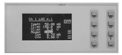
Select the Mode parameter by pushing the (DISPLAY) UP/DOWN ARROW keys until the Mode parameter is highlighted. Repeatedly pushing the (ADJUST) UP/DOWN ARROW keys or turning the ADJUST knob will cycle through the Constant Current low bandwidth (Ilbw), Constant Optical Power (P), Constant Current high bandwidth (Ilbw), and Photodiode Current (Ipd) control modes. Set the LDC-3916330 Series Controller Modules in Constant Current low bandwidth mode by selecting the Ilbw mode.
