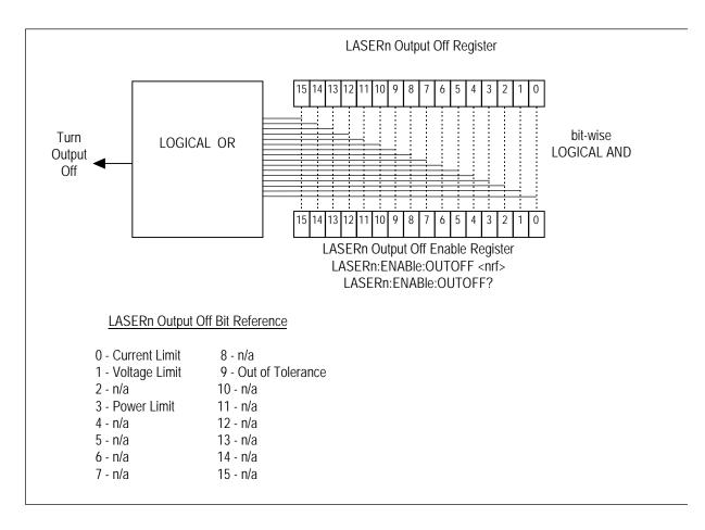
Figure 3.4 LDC-3916330 Series Laser Diode Controller LASER Output Off Register
