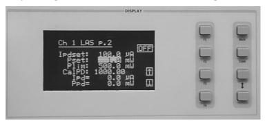
Use the (DISPLAY) UP/DOWN ARROW keys to select the power (Pset) parameter, and adjust the value to 1 mW. The Controller Module will divide the measured photodiode current by the CalPD value to calculate the laser optical power. The current source will automatically adjust the laser drive current to keep the calculated laser power at the Pset value.
