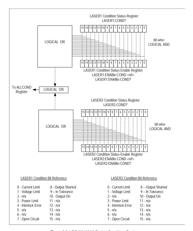
Figure 3.2 LDC-3916330 Series Condition Registers
