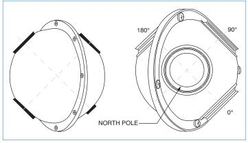
819C 4-Port sphere port locations. Note that a 2" sphere shell is cubic.
