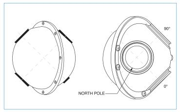
819D 3-Port sphere port locations. Note that a 2" sphere shell is cubic.
