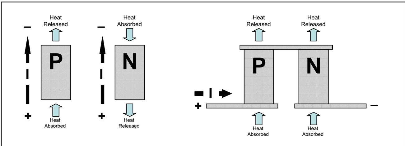
cycle time, it is critical that the TEC is able to swing the device temperature as rapidly as possible.
