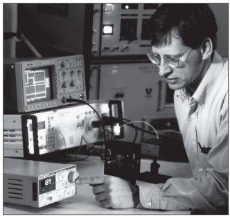
ILX Lightwave instrument designs are subjected to rigorous transient tests. Tests include suppression of 1000V fast-transients and power line surges. (See ILX Lightwave Technical Standard #LDC-00196.)
