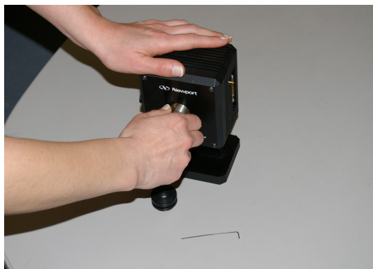
Figure 2. 700-C mount shown with the black protective lens cover and lens cartridge.
