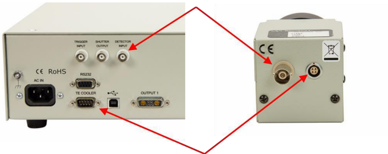
Figure 15 The DETECTOR INPUT and TE COOLER output ports are for direct use of the LIK-LMP with the OPS-Q Power Supply.
