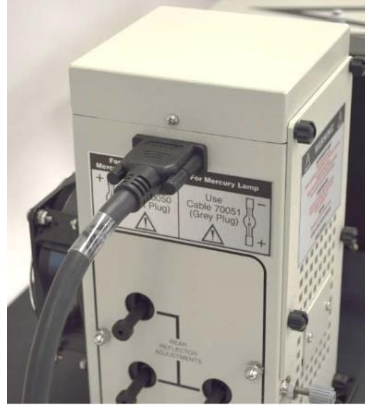
Figure 9 The electrical connector on an Oriel Research Lamp Housing for use with an OPS-Q Model Power Supply.
