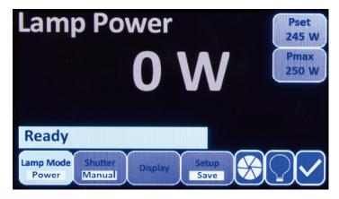
The OPS Series power supplies allow the lamp to be operated in power, current, and intensity control modes.
