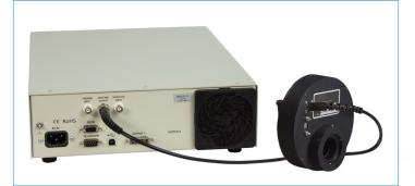
The shutter control feature of the OPS model power supply is useable in power, current, and intensity control modes. Any shutter which responds by opening or closing when receiving a TTL signal can be controlled by the OPS Power Supplies. This includes Oriel's model 71445 low-cost TTL shutter and the shutters designed into the Oriel Solar Simulators.
