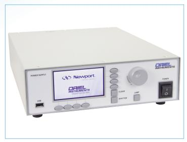
A power switch and all manually controllable features of the OPS model power supplies are accessible from the front panel. Four horizontal push buttons each activate a horizontal menu that allows for configuring of lamp operation mode, shutter, display mode, and setup with the help of a corresponding vertical menu that is activated as well. These functions are conveniently displayed and easily navigated by the LCD display on the front panel of the power supply.
