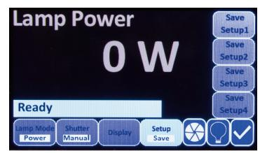
The OPS model power supplies are capable of storing up to four Setups.
