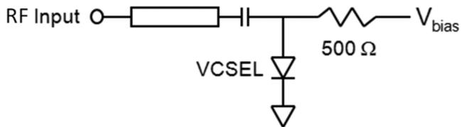
Figure 1. Schematic of VCSEL circuit.
