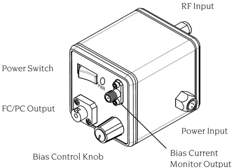
Figure 2. Connector and control descriptions.
