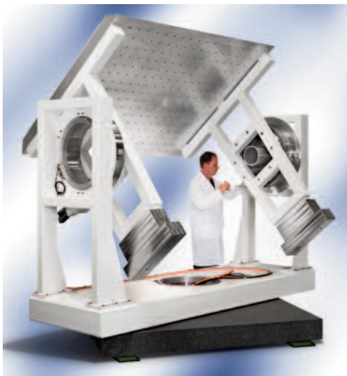
Figure 3: Newport 2-Axis Gimbal for Electro-Optical System Testing
