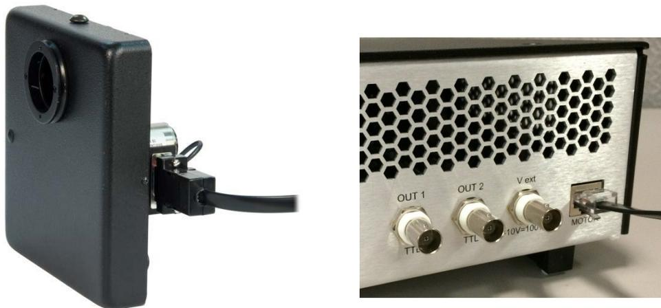
Figure 8: Connecting the Chopper Head to the Controller
