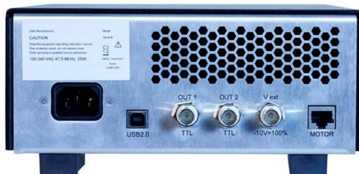
Figure 1: Rear Panel Labels and Warnings
