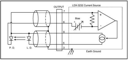
Figure 2.4Common Laser Anode & Photodiode Anode
