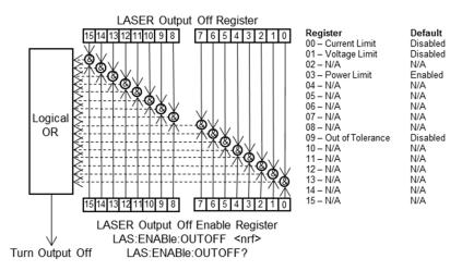
Figure 3.4 LDX-3232 Output Off Register & Defaults
