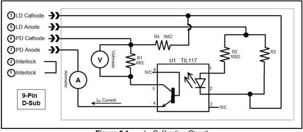
Figure 6.1 I<sub>pn</sub> Calibration Circuit
