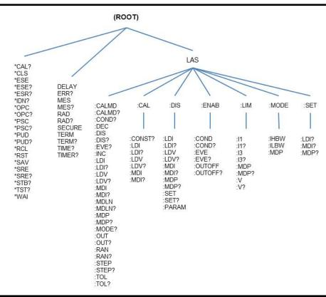
Figure 3.1 LDX-3232 Command Path Structure
