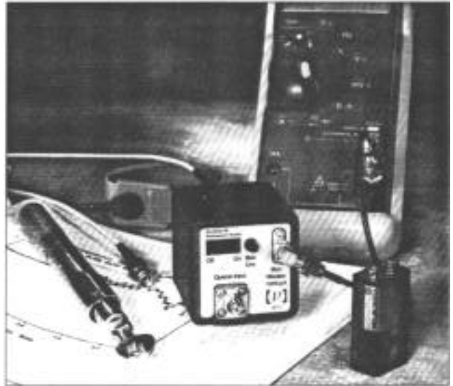
Indium gallium arsenide detector, designed for use in the laboratory, has a 45-GHz bandwidth and operates at wavelengths from 950 to 1650 nm.
