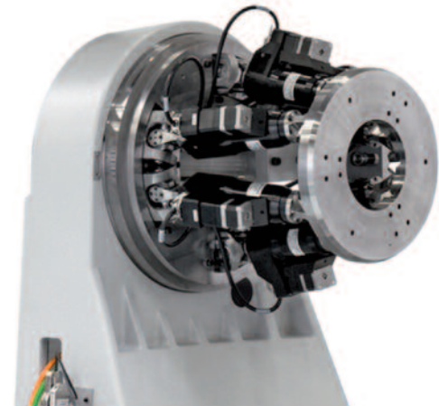
Figure 4: A Hexapod mounted with vertical base configuration on the RVU500 rotary stage
