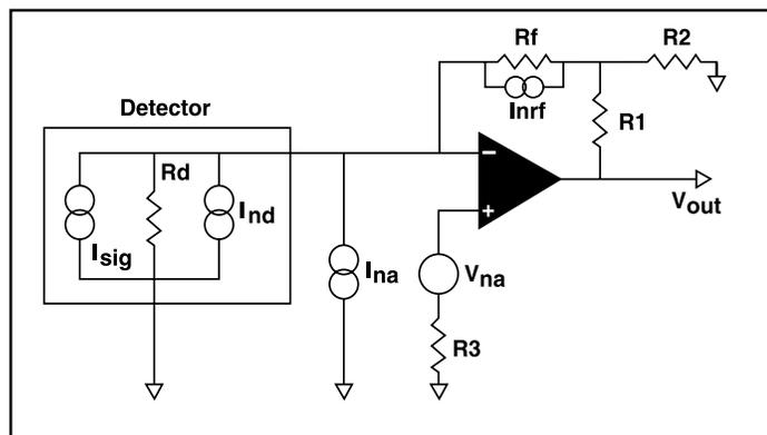
Figure 1. OMH-6709B Receiver Circuit.
