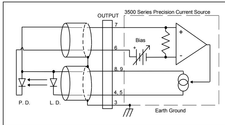
Figure 2.7 Common Laser Anode - Photodiode Anode
