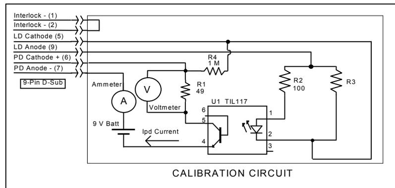
Figure 4.1 IPD Calibration Circuit
