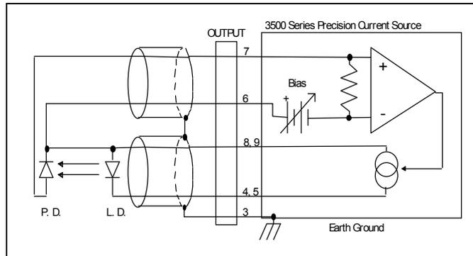
Figure 2.6 Common Laser Anode - Photodiode Cathode
