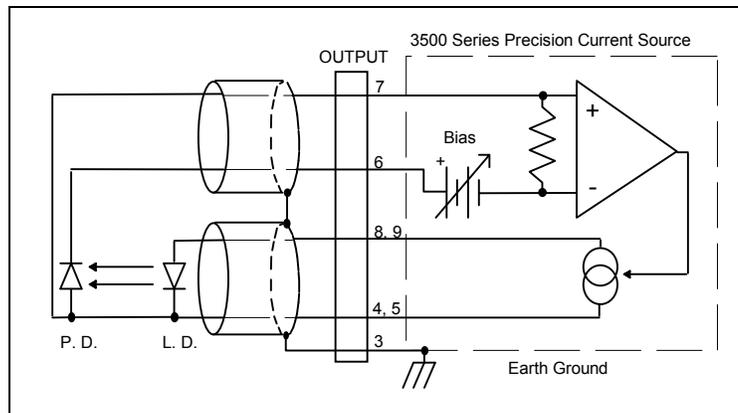
Figure 2.5 Common Laser Cathode - Photodiode Anode
