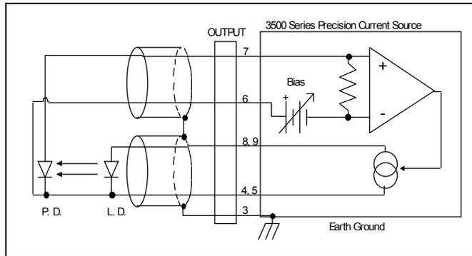
Figure 2.4 Common Laser Cathode - Photodiode Cathode
