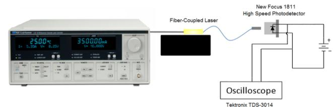
Figure 4: Schematic of transient testing of the LDC-3736 Quantum Cascade Laser Controller
