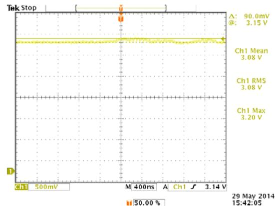
Figure 7: Effect on laser output due to 1 kV power surge event on AC power line
