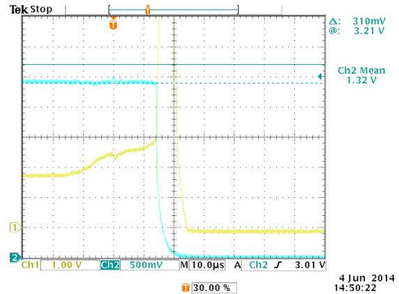
Figure 9: Intermittent contact response of the LDC-3736 with improper voltage limit setting
