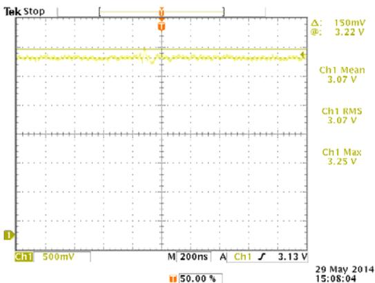
Figure 6: Effect on laser output due to 1 kV EFT event on AC power line
