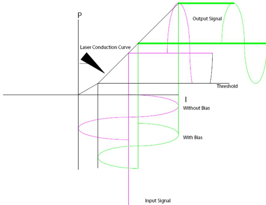
**Figure 1. Modulation of input current and output power.**
