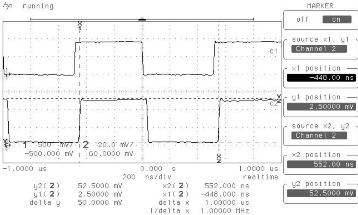
Figure 2. 1 MHz analog modulation for a laser operating at 658 nm.
