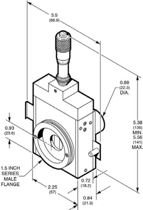
Figure 32: Micrometer Adjustable Slit Dimensions
