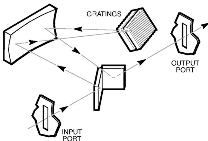
Figure 1: Optical Configuration of the Cornerstone 130
