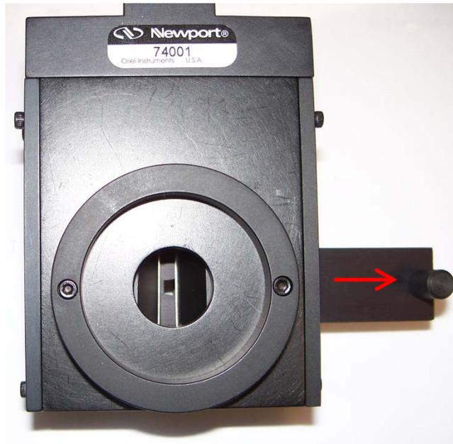
**Figure 11: Shortest Micrometer Adjustable Slit Height**
