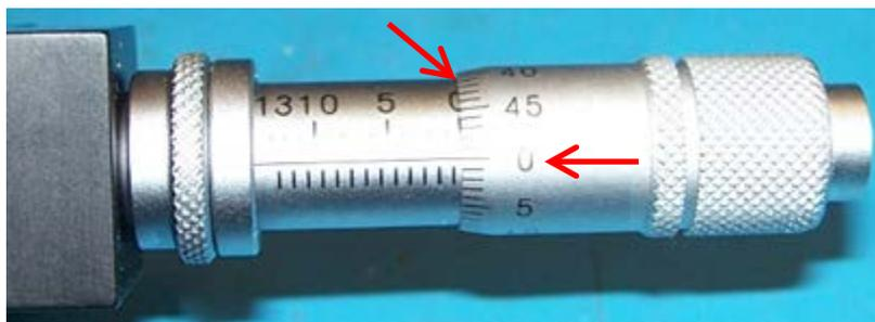
**Figure 10: A Fully Closed Micrometer Adjustable Slit**
