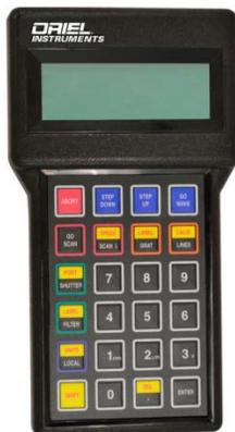
Figure 34: 74009 Hand Controller Keypad
