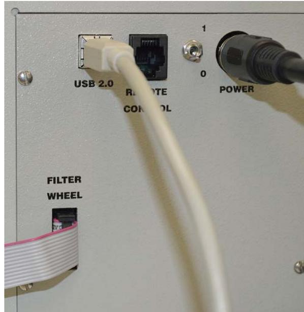
**Figure 6: Monochromator Connections**
