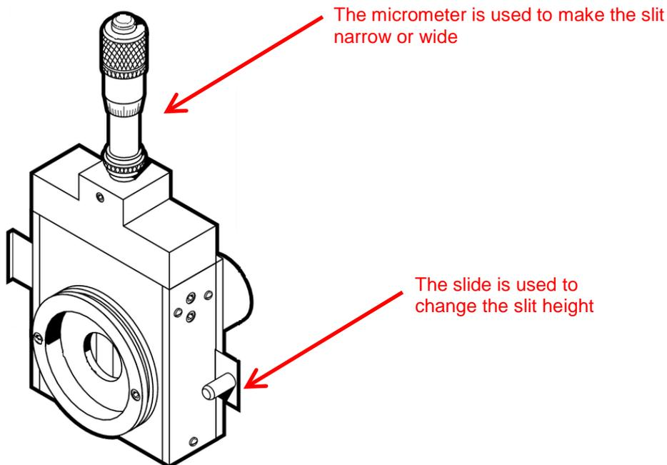
**Figure 9: A Micrometer Adjustable Slit**
