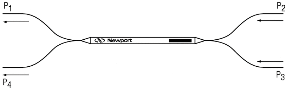
Figure 3. A 1x2 or a 2x2 coupler.
