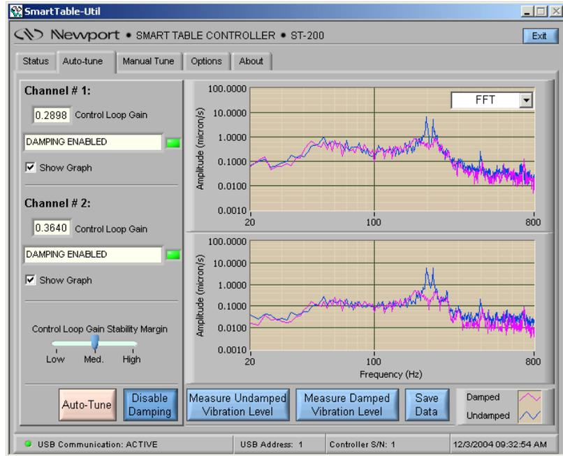
Figure 20 Auto Tune Tab Screen showing dual-channel display
