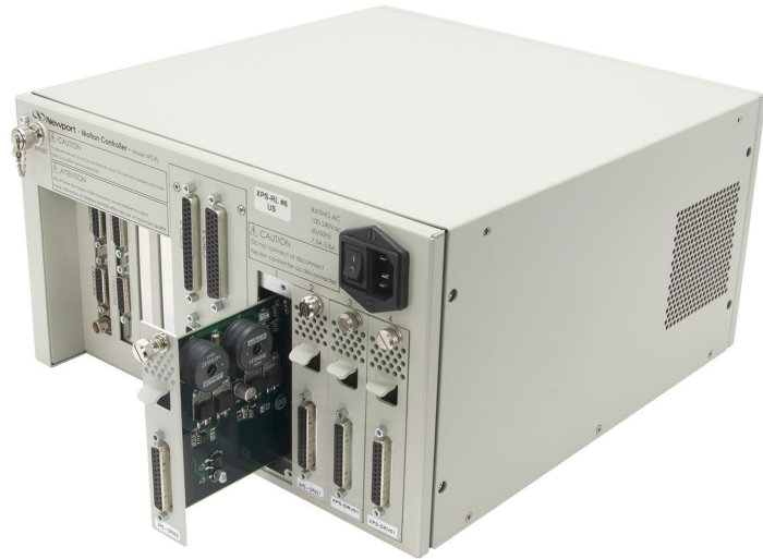
Figure 11: Installing driver cards.
