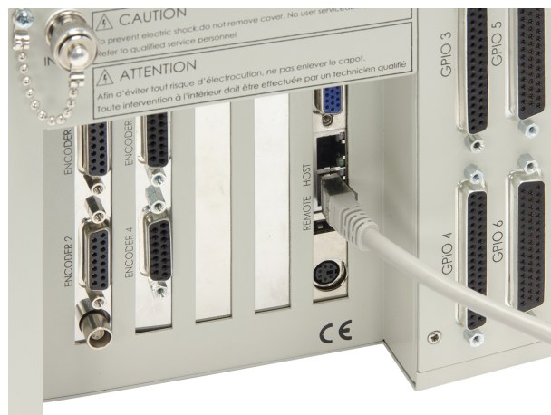
Figure 15: Direct connection to the XPS using a cross-over cable and the REMOTE connector.
