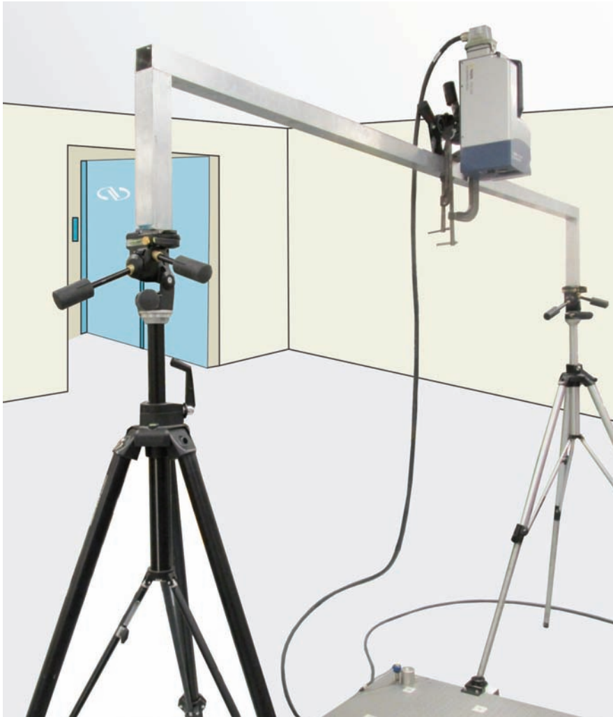
Figure 2. In the test configuration, the laser head was attached to the gantry above the measured surface.
