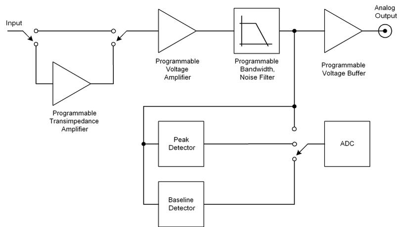
Figure 64 Model 1936/2936 Series Analog Signal Flow Diagram
