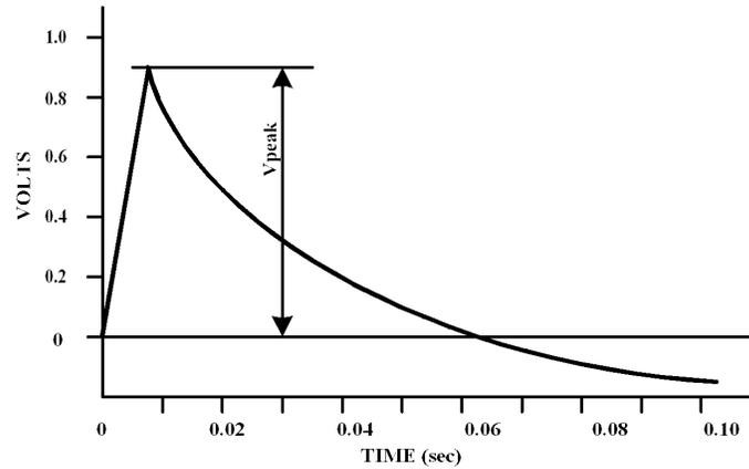
*Figure 66 Typical Newport Energy Detector Signal Waveform*
