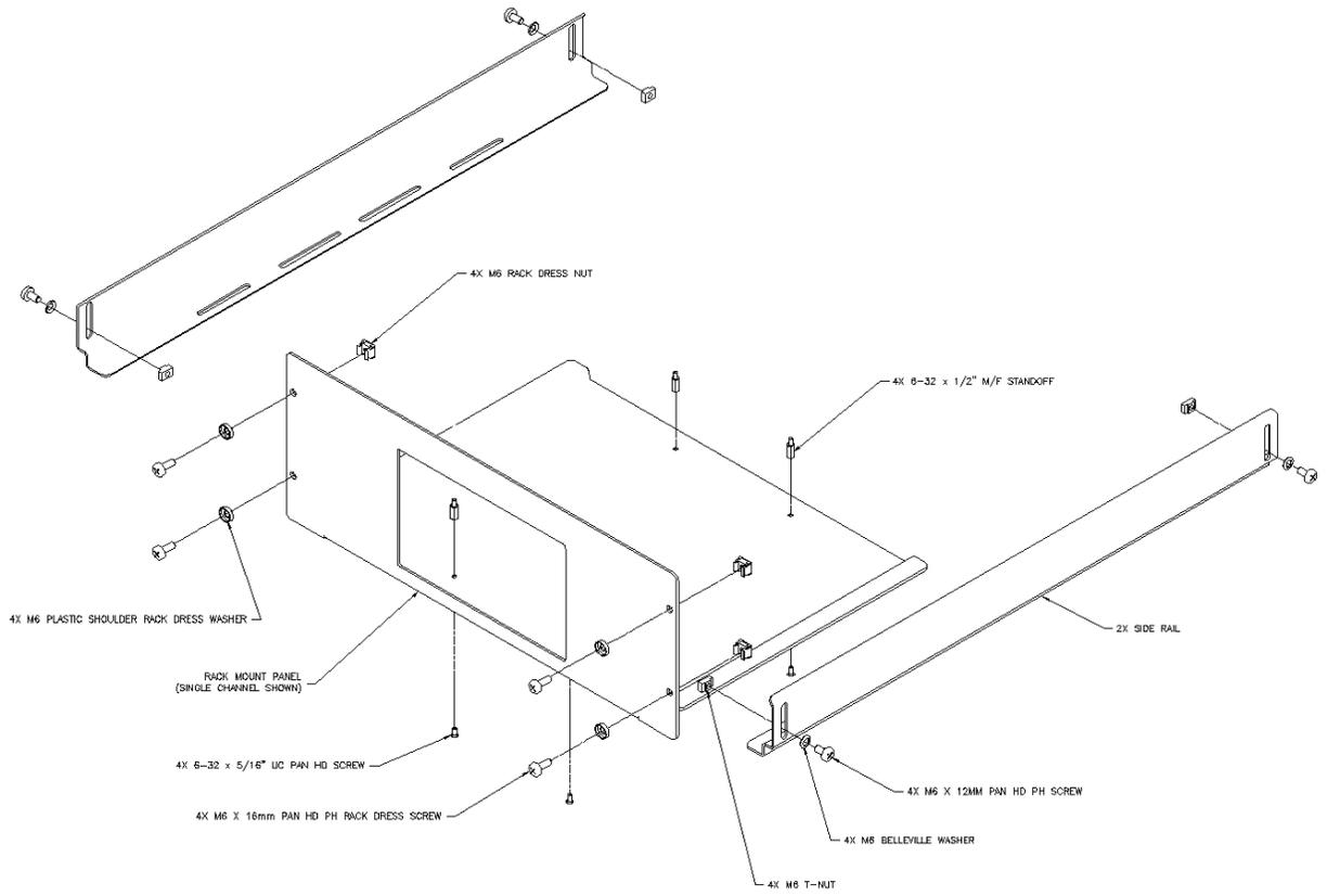
Figure 20 Mounting details for the PMI-RACK mounting kit
