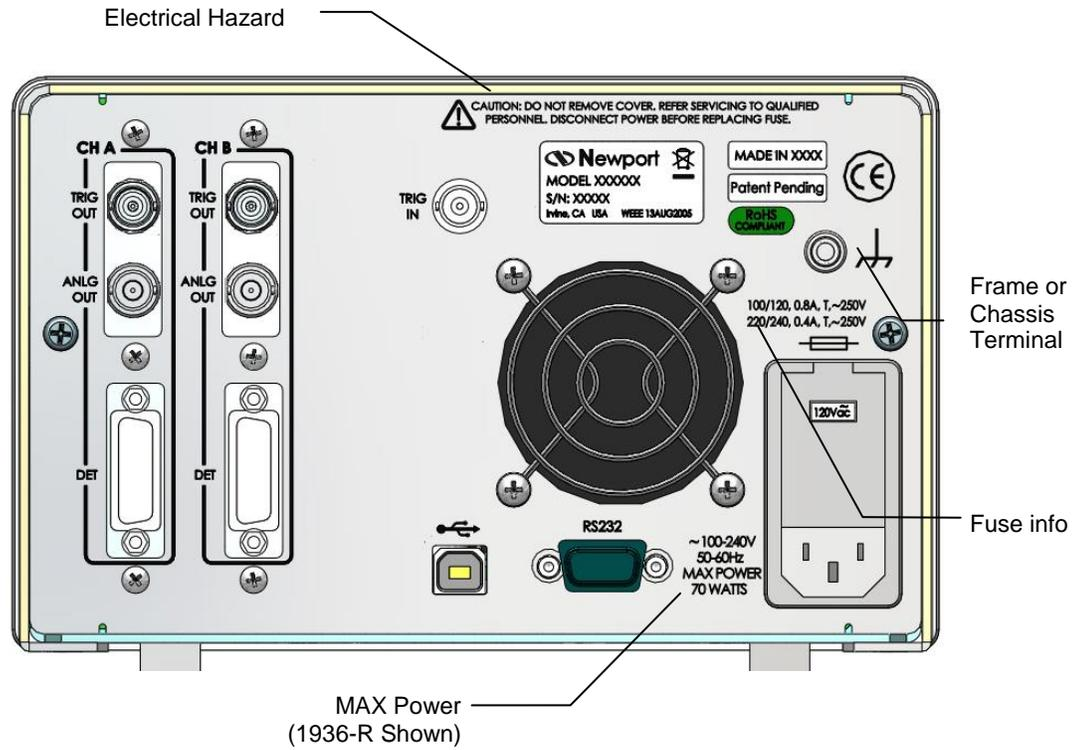
Figure 14 Locations of warnings on the rear panel
