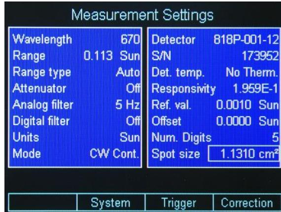
Figure 25 Measurement Settings screen
