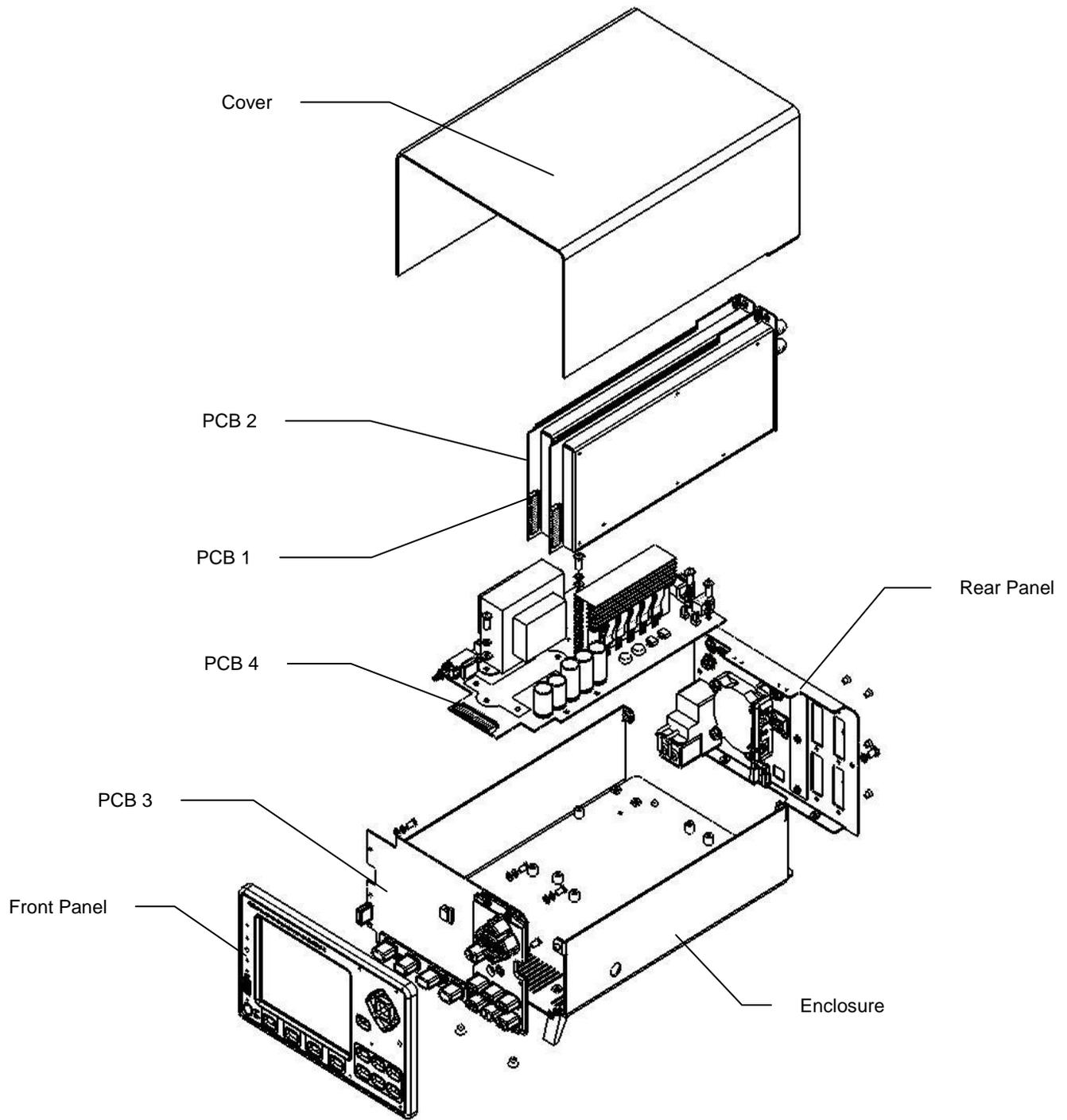
Figure 72 Disassembled 1936/2936 model
