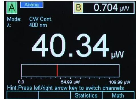
Figure 57 Analog Needle display
