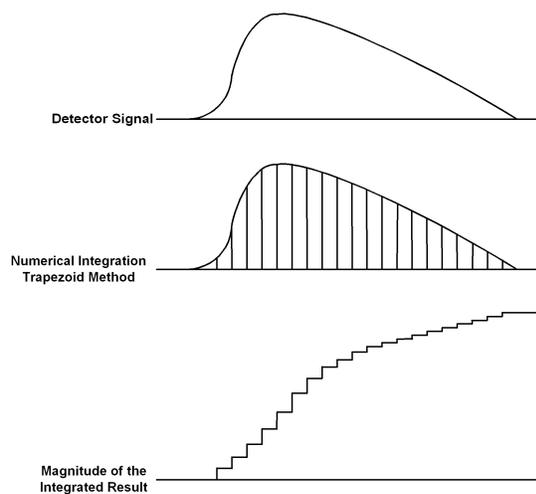
Figure 69 Integrated Energy Via a Trapezoid Approximation.
