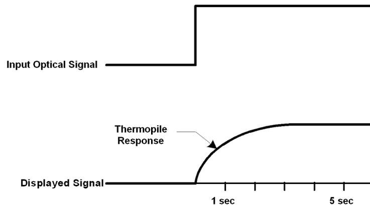
Figure 65 Thermopile Signals exhibit 1 to 10 second time constants.
