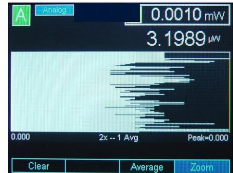
Figure 59 Vertical chart with 1 measurement per line
