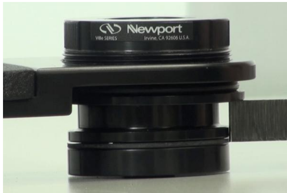
Figure 11 Gap tool thickness measurement showing correct preload.
