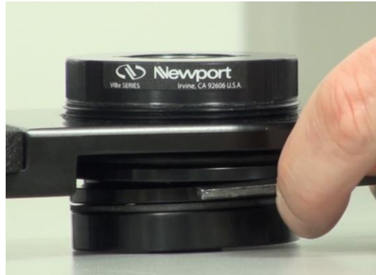
Figure 10 Gap tool thickness measurement showing overloaded condition
