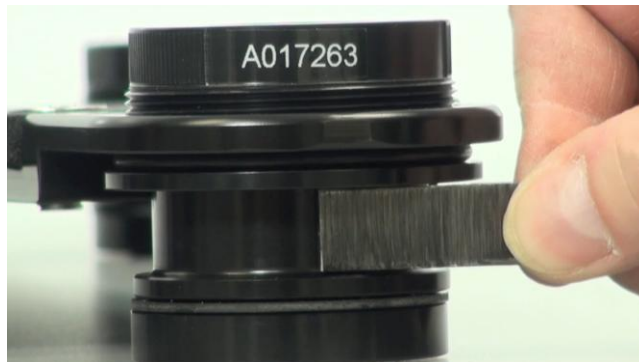
Figure 9 Gap tool width measurement showing under loaded condition
