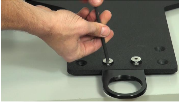
Figure 3 Mounting the VIB-BRKT to the base plate
