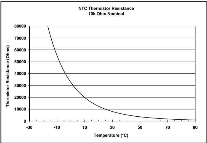
Figure 2 10kW Thermistor Curve
