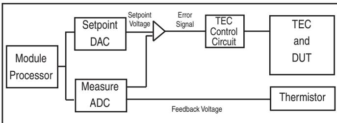
Figure 1 Temperature Control Circuit / Feedback Loop
