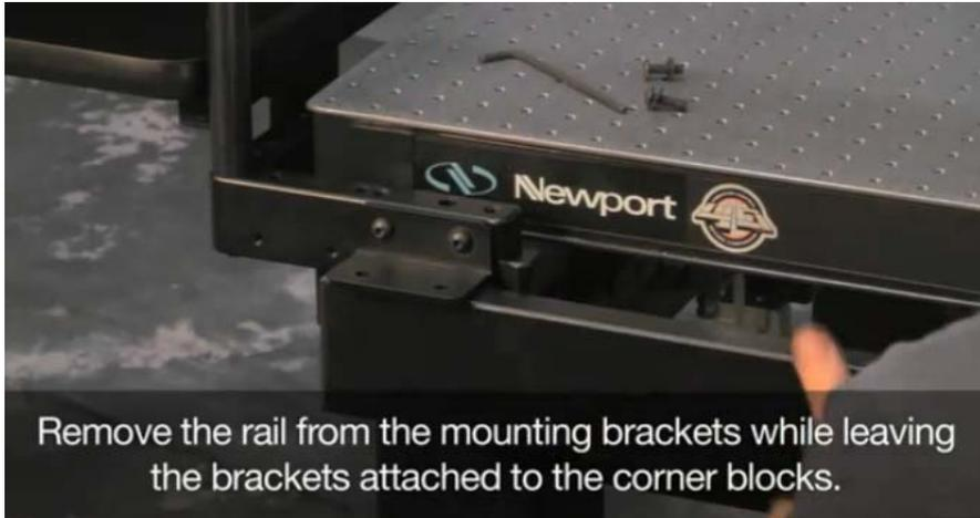
Remove the rail from the mounting brackets while leaving the brackets attached to the corner blocks.
