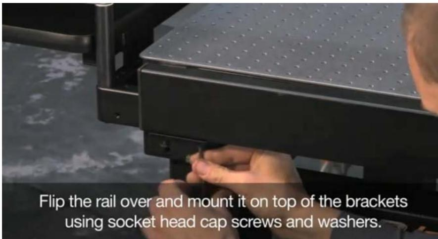
Flip the rail over and mount it on top of the brackets using socket head cap screws and washers.
