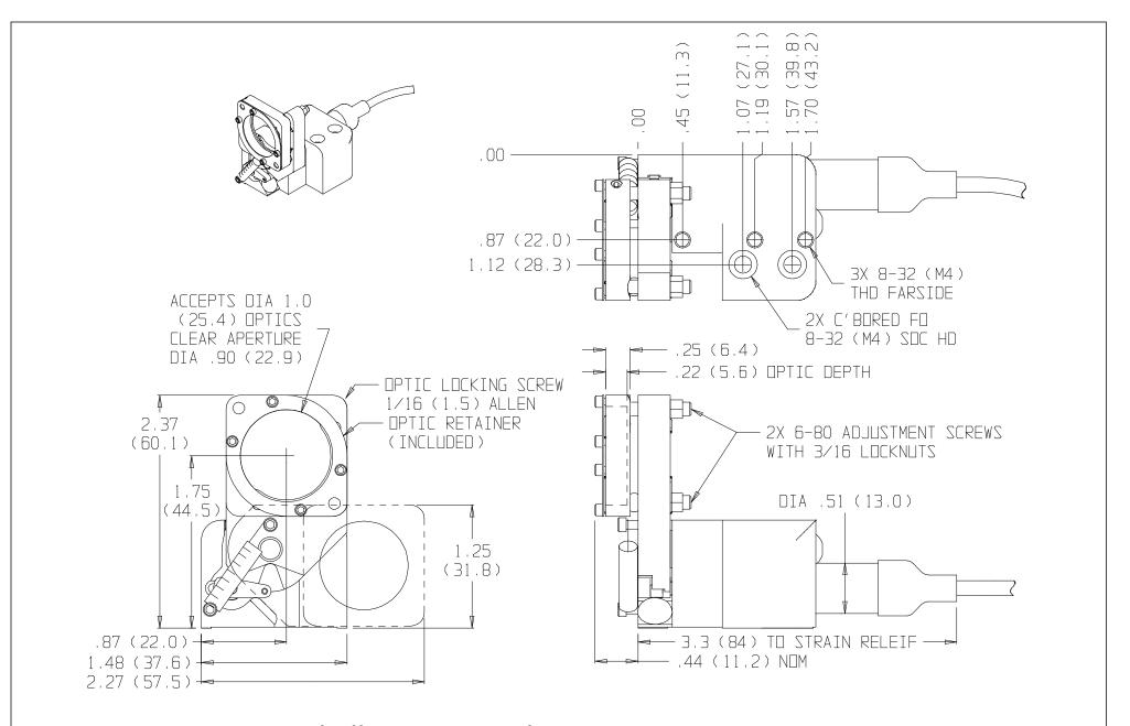
8892-K Motorized Fllipper Optical Mount
