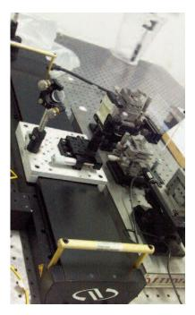
With its broad domain of applications, fiber grating technology has inspired researchers to continue the investigation of its property and optimization of technique. Many researchers often develop their own experimental setup to fabricate the fiber gratings, and the image shows an example using Newport stage. This setup is a phase mask inscription system which consists of a UV laser (not shown), Cylinder lens, high precision motorized linear stages and phase mask.
