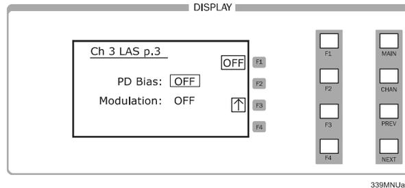
**Figure 2.7** Modulation On/Off Screen, Laser Page 3
