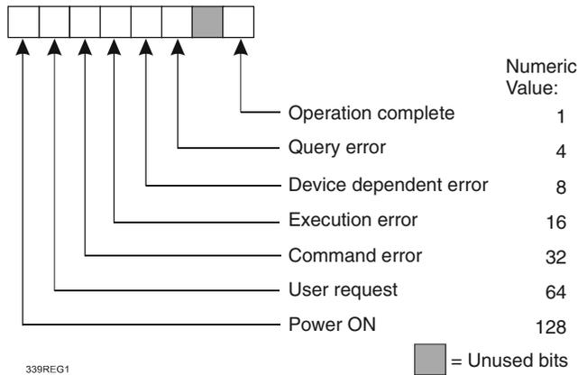
Notes Bit 5 of the status byte register is set if any enabled conditions are true.
