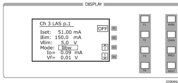
Figure 2.6 Constant Current Mode Setup, Laser Page 1
