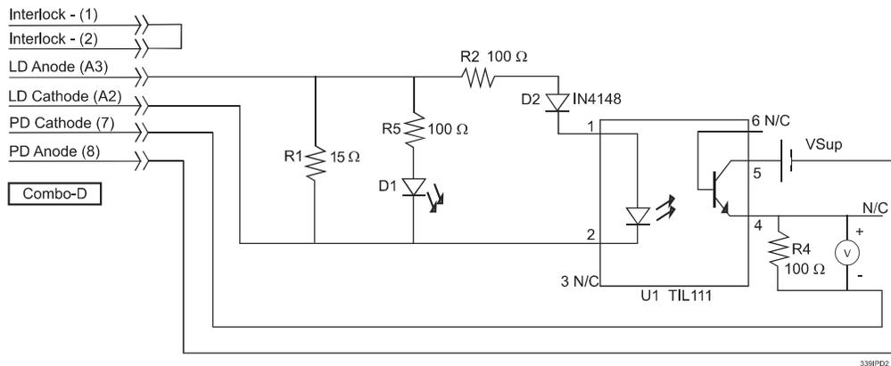
**Figure 5.1** I<sub>PD</sub> Calibration Circuit
