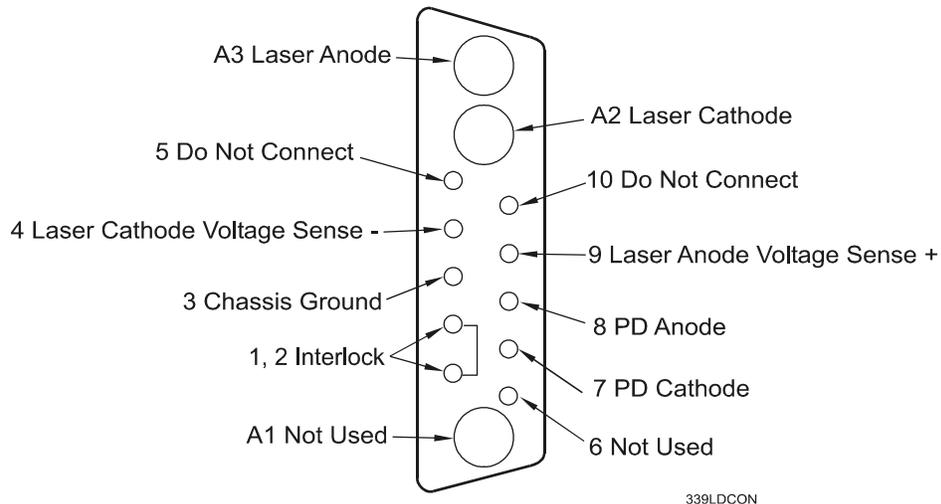
**Figure 2.2** Back Panel Laser Diode Connector
