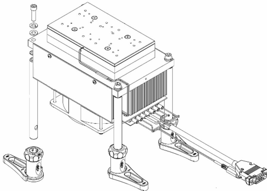
Figure 6 Model 764H-110 mounting hardware and electrical connections
