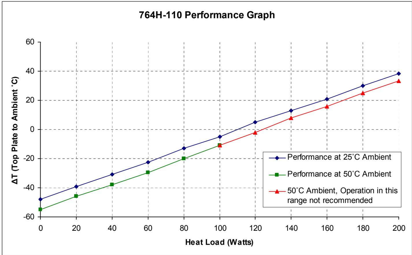
Figure 4 Model 764H-110 heat removal performance chart
