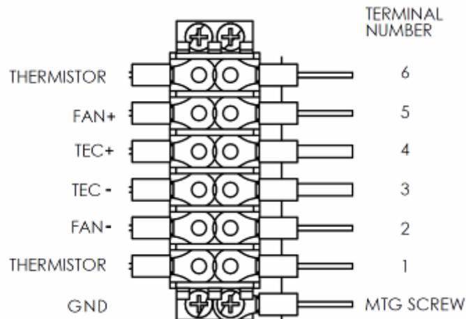
Figure 14 Terminal block connections
