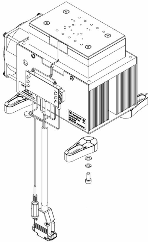
Figure 5 Model 764H-061 mounting hardware and electrical connections
