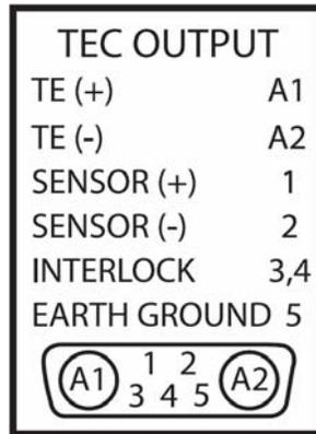
Figure 15 Pinout of cable for models 3150 and 3700
