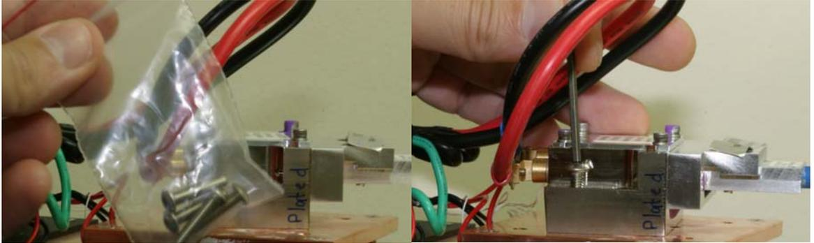
Figure 11 Mounting screws for BWA series LD
