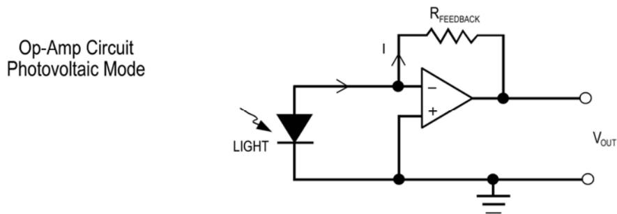
Figure 4 Newport detector circuitry used in photovoltaic mode
