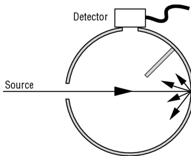
Figure 3 819C integrating sphere configuration.
