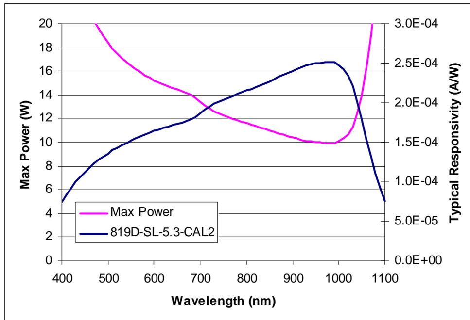
Figure 5 Typical responsivity curve of 819D-SL-5.3-CAL2
