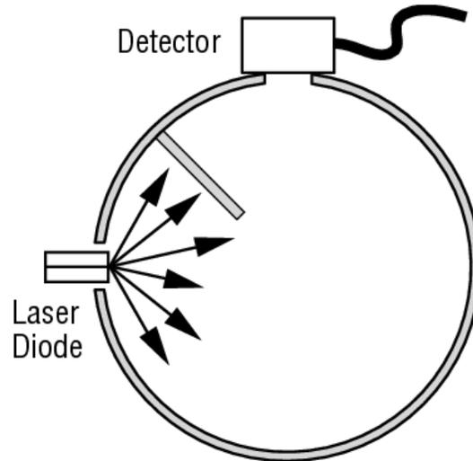
Figure 2 819D integrating sphere configuration.
