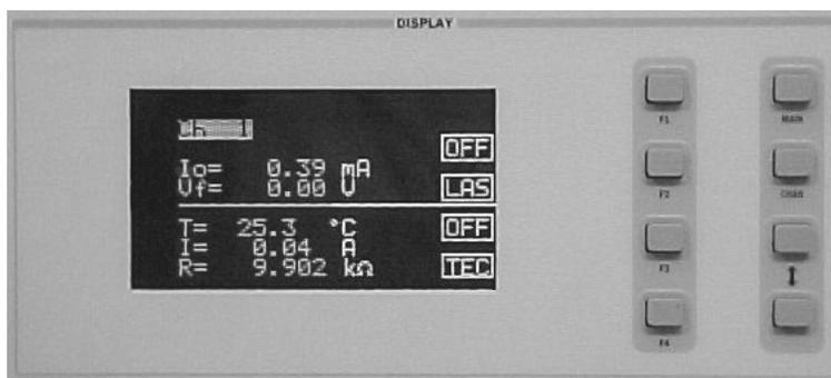
To enter the setup menu, push the CHAN key, which displays the channel menu. Select the correct channel number at the top of the display by pushing the (ADJUST) UP/DOWN ARROW keys or turning the ADJUST knob. Then push the DISPLAY LAS soft key (F2) to enter page 1 of the laser setup menu.
