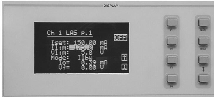
Now select the current limit (Ilim) parameter using the (DISPLAY) UP/DOWN ARROW keys. Adjust the value to 175mA. The current limit protects your laser by never allowing the laser drive current to exceed the Ilim value independent of the current set point and the controller mode (Constant Current or Constant Power).
