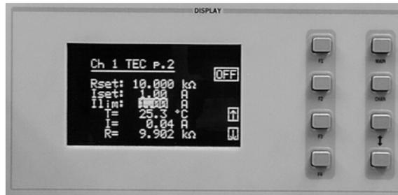
To set the TEC current limit to 1.5 Amps, first select TEC p. 2 by pushing the down soft key (F4) on the TEC p. 1 menu. Use the (DISPLAY) UP/DOWN ARROW keys to highlight the ILim value. Next, use the (ADJUST) UP/DOWN ARROW keys, knob, or the keypad to enter the desired value of 1.5 amps (A).
