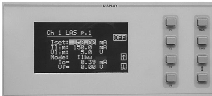
Next, select the Iset parameter on the setup menu using the (DISPLAY) UP/DOWN ARROW keys. This parameter sets the laser current source drive value when in Ilbw or Ihbw modes. Enter 150 mA using the numeric keypad, the ADJUST knob, or the (ADJUST) UP/DOWN ARROW keys. Push the ENTER key to store the value in memory within three seconds after entering the value using the numeric keypad, or it will revert to the old value.
