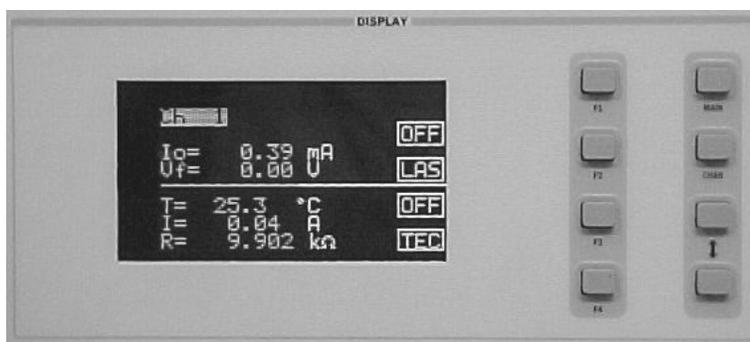
Push the CHAN key to display the single channel menu. From this menu you can see the measured parameters, enter the LAS or TEC channel setup menus, or turn the LAS current source and/or TEC on and off. Use the (ADJUST) UP/DOWN ARROW keys or the ADJUST knob to select the desired channel number highlighted at the top of the display. Push the DISPLAY LAS soft key (F2) to enter page 1 of the laser channel setup menu.
