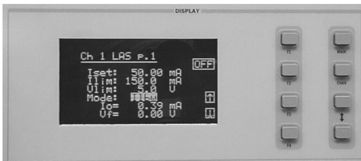
Select the Mode parameter by pushing the (DISPLAY) UP/DOWN ARROW keys until the Mode parameter is highlighted. Repeatedly pushing the (ADJUST) UP/DOWN ARROW keys or turning the ADJUST knob will cycle through the
