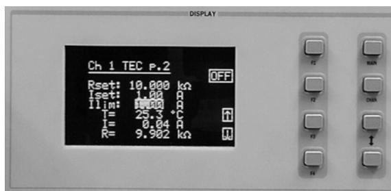
To adjust the GAIN value, first select TEC p.3 by pushing the down soft key (F4) on TEC p.2. Then use the (DISPLAY) UP/DOWN ARROW keys to highlight the GAIN number. To change the value, use the (ADJUST) UP/DOWN ARROW keys, knob, or the keypad to enter the desired value. The quickest way would be to use the keypad for large changes in gain values. Set the temperature control loop GAIN value to 30.
