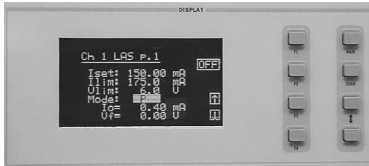
Select the Mode parameter by pushing the (DISPLAY) UP/DOWN ARROW keys until the Mode parameter is highlighted. Repeatedly pushing the (ADJUST) UP/DOWN ARROW keys or turning the ADJUST knob will cycle through the Constant Current low bandwidth (Ilbw), Constant Optical Power (P), Constant Current high bandwidth (Ihbw), and Photodiode Current (Ipd) control modes. Set the LDC-3916370 Series Controller Module in Constant Optical Power mode by selecting the P mode.
