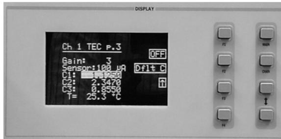
To adjust the value of a C1, C2, or C3 constant, use the (DISPLAY) UP/DOWN ARROW keys to highlight the desired constant name (C1, C2, or C3). To change the value, use the (ADJUST) UP/DOWN ARROW keys, knob, or the keypad to enter the desired value. The range of values for C1, C2, and C3 are -99.9999 to +99.9999. The quickest way would be to use the keypad for large changes in constant values.
