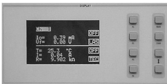
To access any of the TEC Control setup menus, you must start with the channel menu. This can be accomplished in several ways; the most direct way is to depress the CHAN hard key right below the MAIN key. Here you can select the desired channel by turning the (ADJUST) knob or pushing the (ADJUST)
