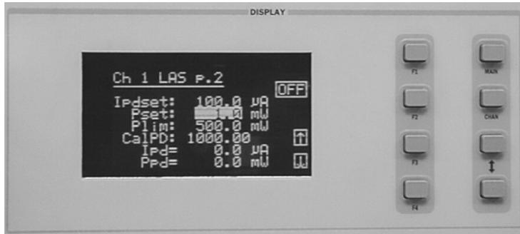
Use the (DISPLAY) UP/DOWN ARROW keys to select the power (Pset) parameter, and adjust the value to 1 mW. The Controller Module will divide the measured photodiode current by the CalPD value to calculate the laser optical power. The current source will automatically adjust the laser drive current to keep the calculated laser power at the Pset value.
