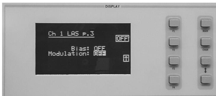
The Modulation parameter on the LAS p.3 setup menu controls whether the MODULATION connector input is active or not. Select the Modulation parameter by pressing the (DISPLAY) UP/DOWN ARROW keys until the Modulation parameter is highlighted. Adjust the value to ON or OFF as desired. Refer to the LDC-3916370 Series module specifications in Chapter 1 for modulation input specifications and limitations.
