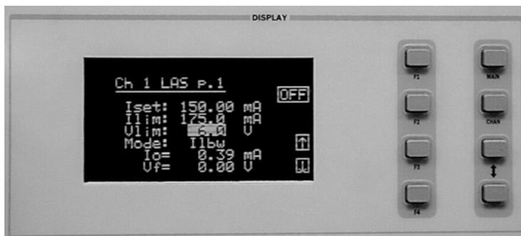
Next, select the laser voltage limit (Vlim) parameter using the (DISPLAY) UP/DOWN ARROW keys. Adjust this value to your desired laser voltage limit. The voltage limit also protects your laser by shutting off the source driver if the laser voltage exceeds the Vlim value. The Vlim value should be set slightly above the operating voltage of the laser diode to provide maximum protection.
