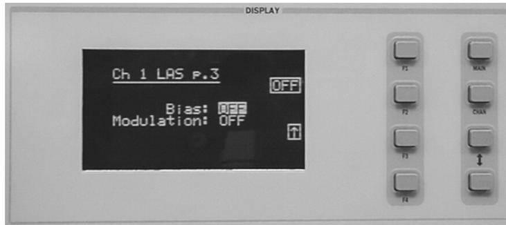
The Bias parameter setting controls whether a 5 volt reverse voltage is supplied to the monitor photodiode or not. Set the Bias parameter to ON or OFF as desired.
