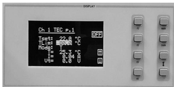
To set the temperature limit to 40°C, use the (DISPLAY) UP/DOWN ARROW keys to highlight the TLim value. Next, use the (ADJUST) UP/DOWN ARROW keys, knob, or the keypad to enter the desired value of 40°C.
