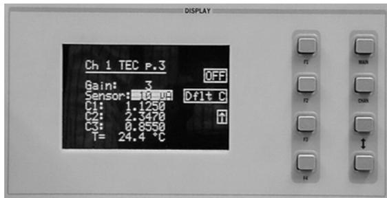
To set the temperature controller's Sensor range, use the (DISPLAY) UP/DOWN ARROW keys until the SENSOR parameter is highlighted. Repeatedly pushing the (ADJUST) UP/DOWN ARROW hard keys or turning the ADJUST knob will cycle through the available thermistor current modes of 100  $\mu$ A and 10  $\mu$ A. Set the temperature controller in 100  $\mu$ A sensor range.
