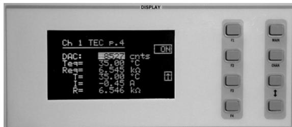
Set the TEC menu to page 4. The DAC value may be adjusted by using the (ADJUST) UP/DOWN ARROW hard keys, knob, or by entering in the value on the keypad. As the DAC value changes, the equivalent temperature and resistance are calculated and displayed beneath the DAC value.
