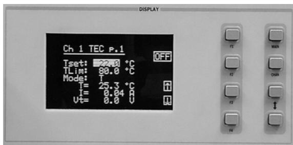
To adjust the Temperature Set Point to 25°C, use the (DISPLAY) UP/DOWN ARROW key to highlight the Tset value. Next, use the (ADJUST) UP/DOWN ARROW keys, knob, or the keypad to enter the desired value of 25°C.
