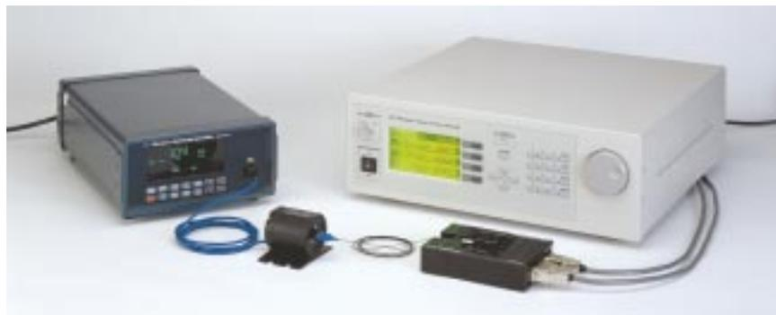
FIGURE 2. Modular laser-diode controller (Newport Model 8008) characterizes fiber-pigtailed laser diodes for telecommunication. This controller can drive and control temperature for up to eight lasers. Sixteen devices can be operated simultaneously if temperature-control capability is not required.
